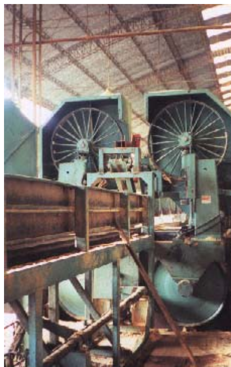
Plate 5 : Twin band head-rig for primary log reduction
