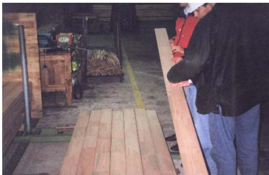
Plate 3 : Inspecting finger jointed E. grandis flooring
