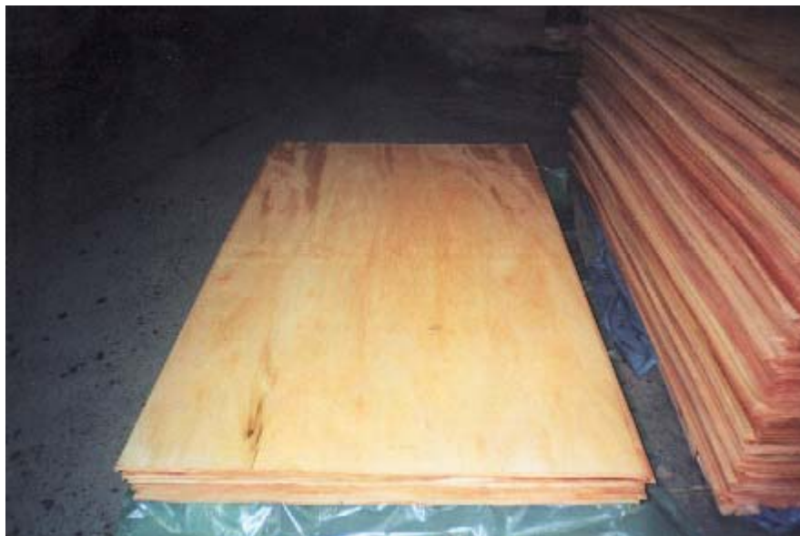
Plate 9 : Rotary peeled E. grandis veneers
