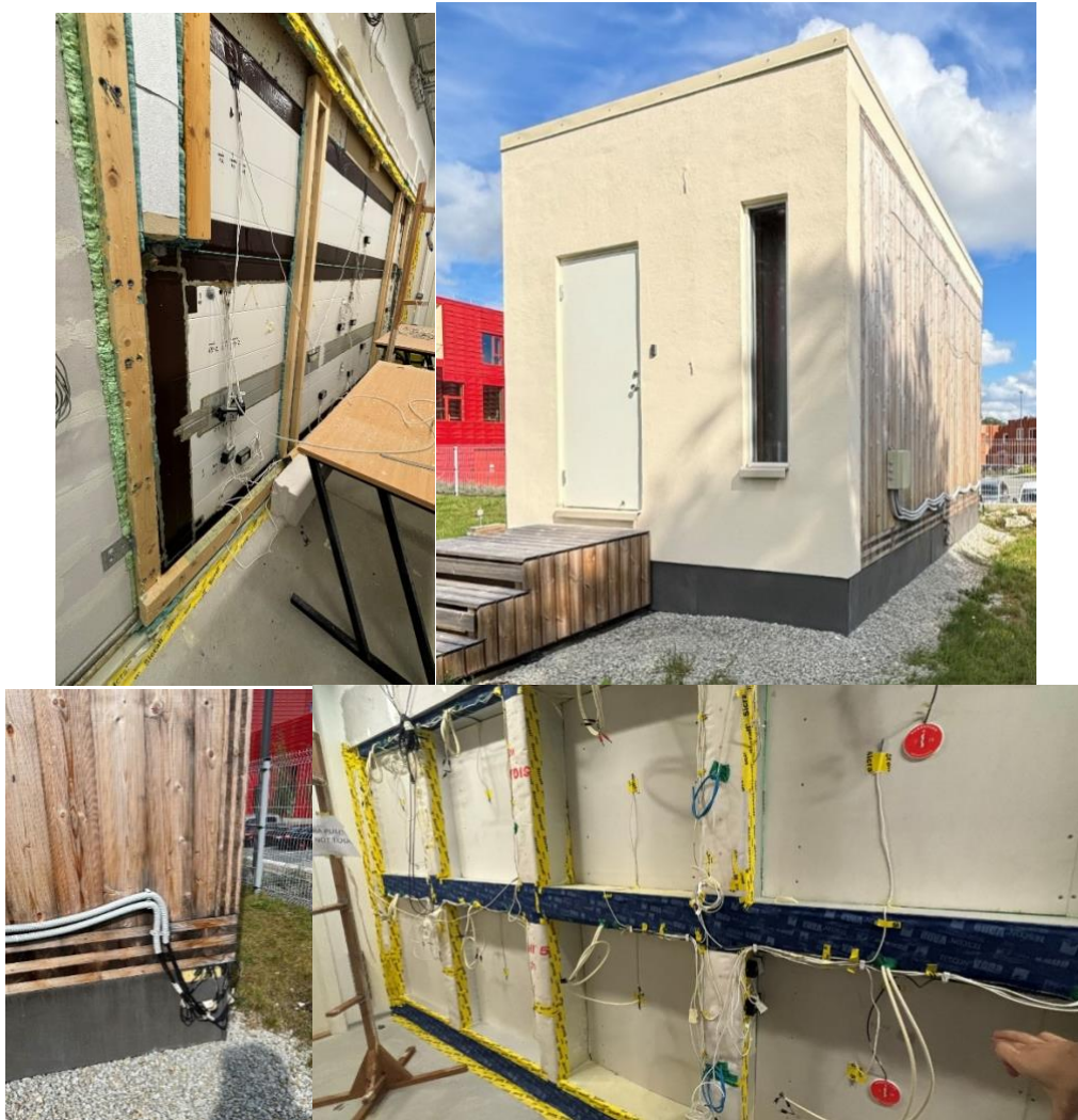
Figure 13: Large scale experimental set up at TalTech testing the moisture changes in timber structures (CLT and timber framing) using real-time data collection.
