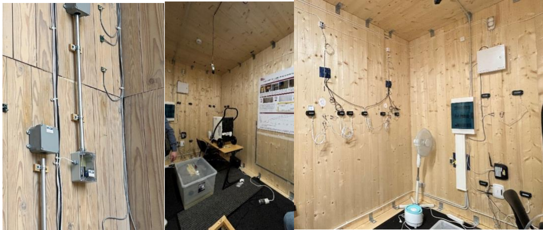
Figure 14: Large scale indoor and outdoor condition monitoring of timber structures using different types of sensors at TalTech.
