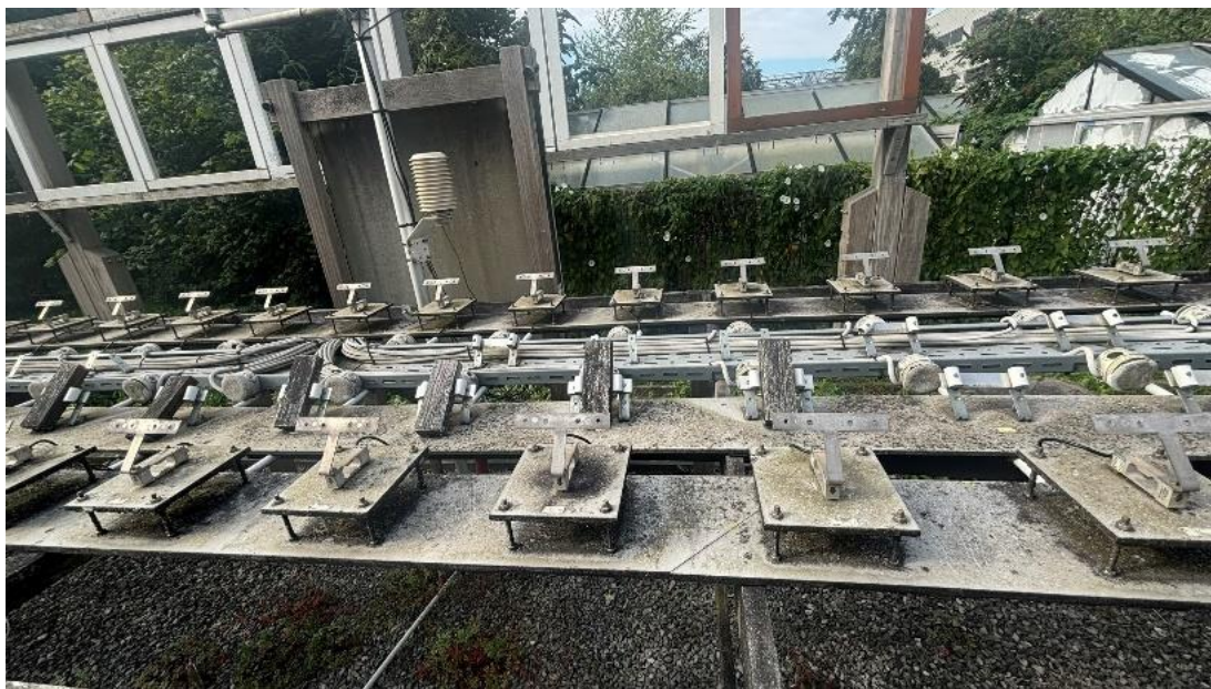
Figure 7: Field trial set up at the University of Ghent monitoring continuous moisture changes of timber sections exposed to weather.
