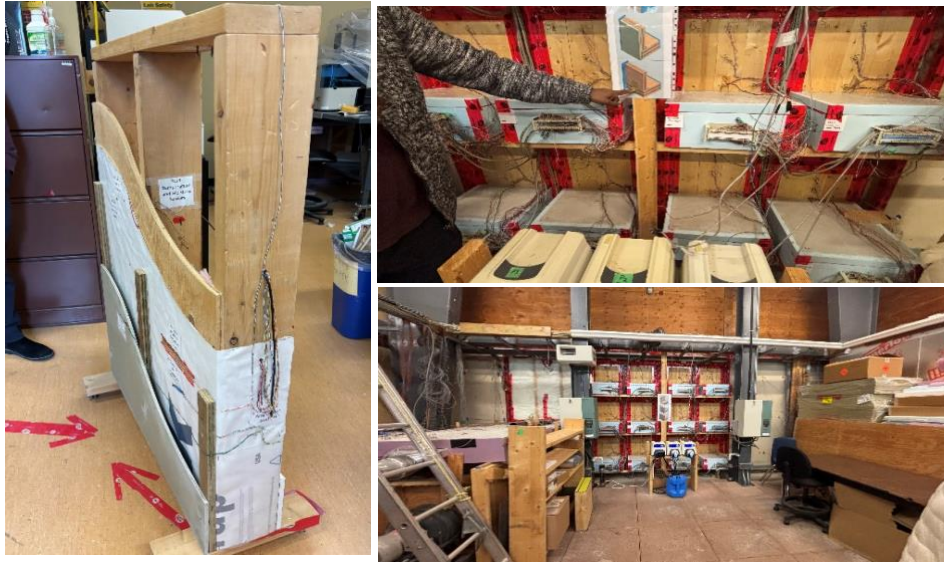
Figure 11: Laboratory study of building sections exposed to various moisture scenarios.
