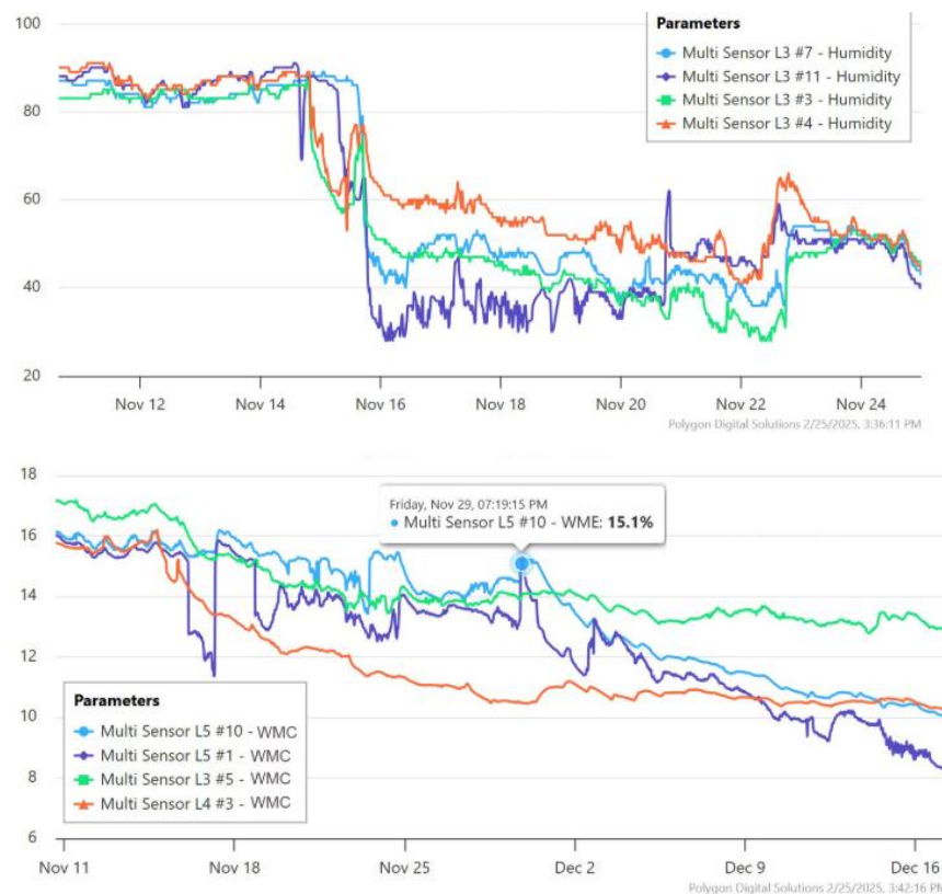
Figure 20: Monitoring of drying panels using desiccant drying technology in a case study building exposed to prolonged rain and water pooling [35].
