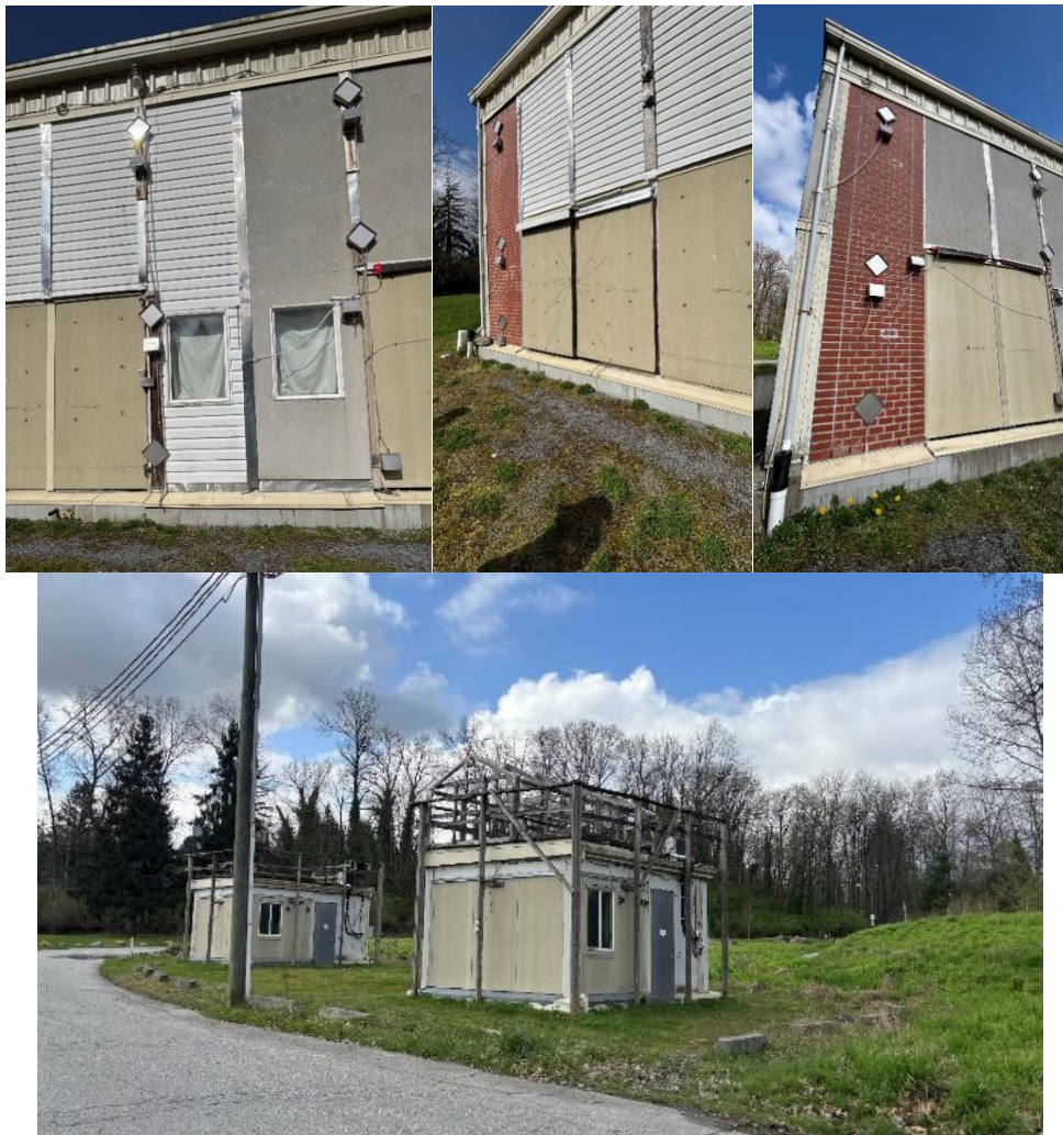
Figure 12: Large scale testing of timber building section set up with different layer up exposed to post-construction (leak/condensation) moisture.
