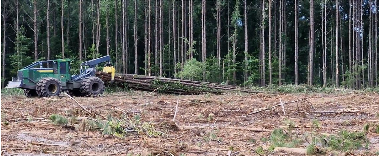
Figure 6 Skidder Transporting Bunched Loblolly Pine
