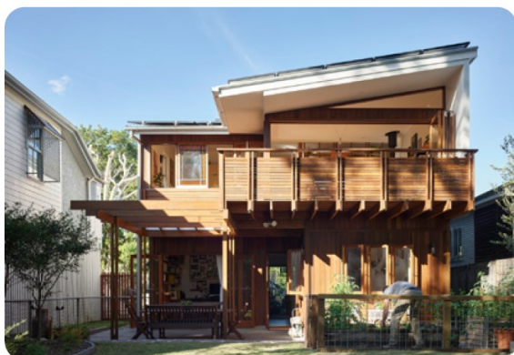
The Chelmer Flood House designed by JDA Co. is an existing Queensland house that had a history of riverine flooding that was renovated and extended with a flood-resilient design. It’s currently a model for the “Design guidance for flood resilient homes” issued by the Queensland Government.
