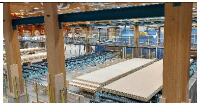
Lamellae are glued together with PUR adhesive.
