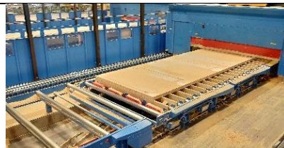
Lamellae are pressed to form large plates.
