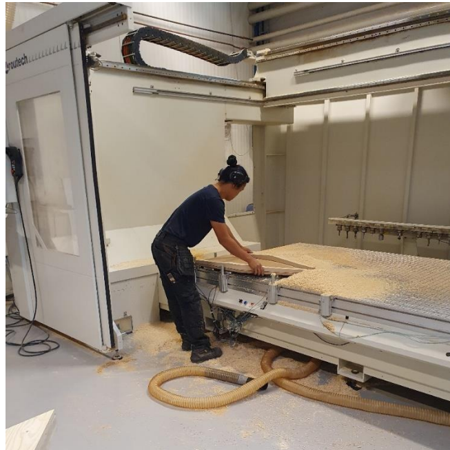
Figure 9 A Stenebyskolan student loads a CNC machine with chair legs to be shaped. The chair legs are produced by the students for a “real” external client (a local furniture manufacturer).
