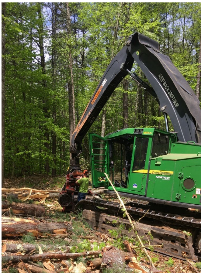
Figure 15 - Maintaining the chain of a processor head on a cut to length operation.
