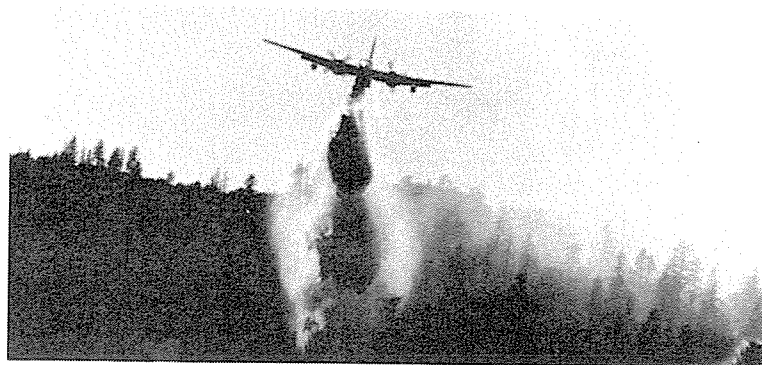
Figure 14: P2 Neptune Air Tanker Bomber releasing 2000 US Gallons of retardant to back up the boundary of a back burning operation. Savage Fire, near Mariposa, Central California. September 1990.
