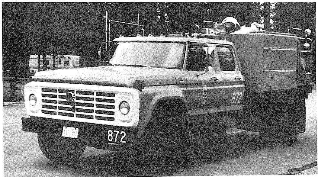
FIGURE 13: Standard sized USDA Forest Service Fire Engine. Seating Capacity 5, water capacity, 250 US Gallons.
