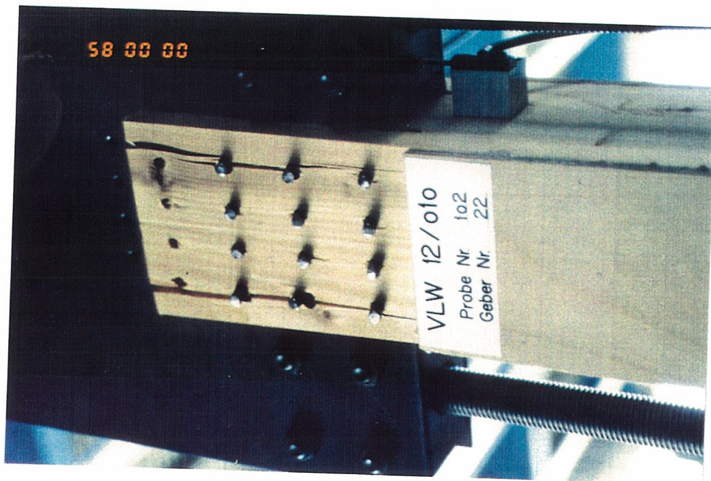
Photograph 2.6 - Load duration (creep) testing of high axial loaded connections
