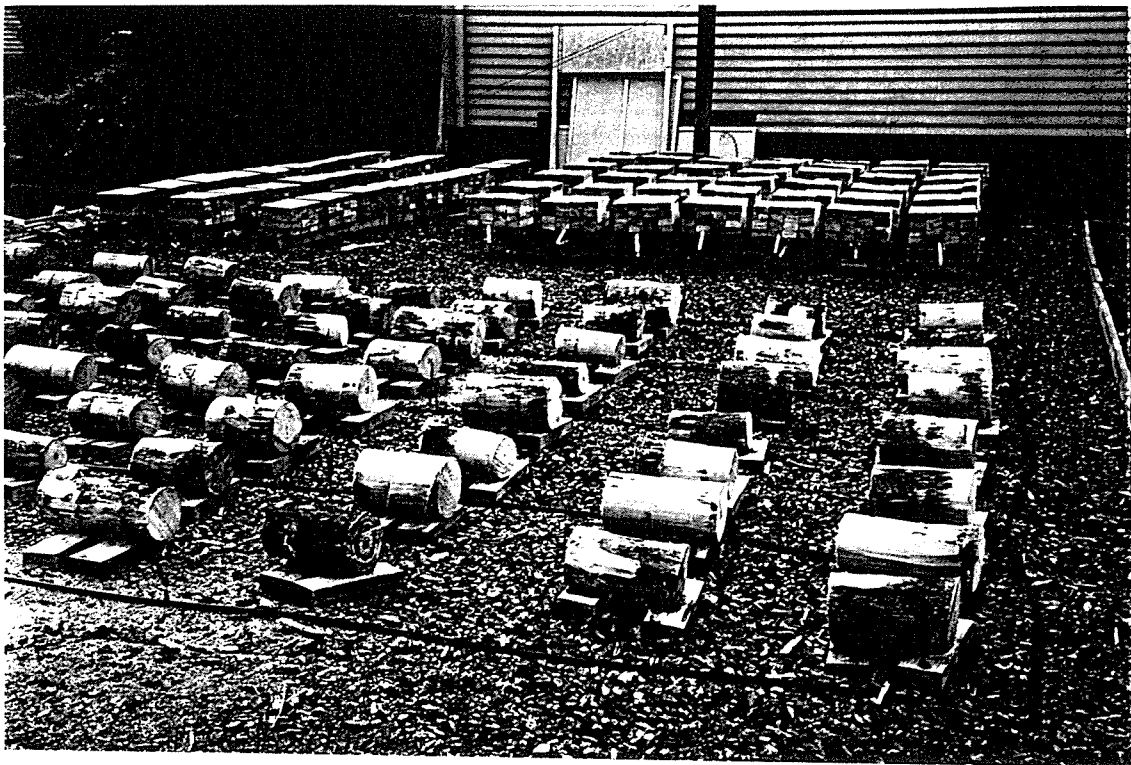
An example of a small scale field trial to test effectiveness and weathering of potential biological control preparations. Both block stacked timber and roundwood are used for visual assessment.
