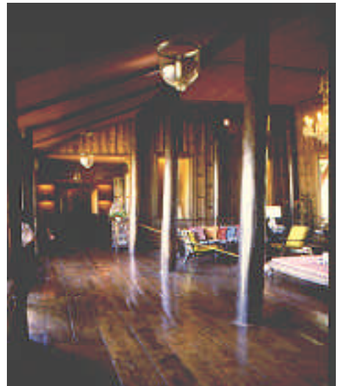
Below: external cladding is reused inside the building and reversed to give scale and texture. The modular system allows for bays to be cut into the panels in a visually acceptable manner.
