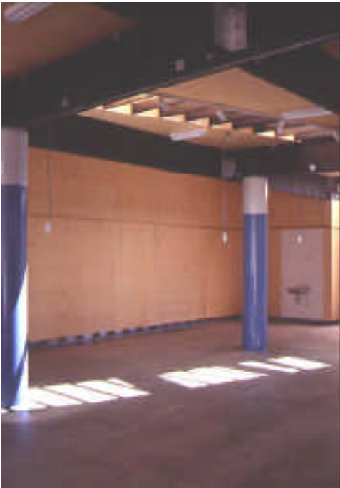
Above: roof lighting gives additional natural light saving on energy consumption.
