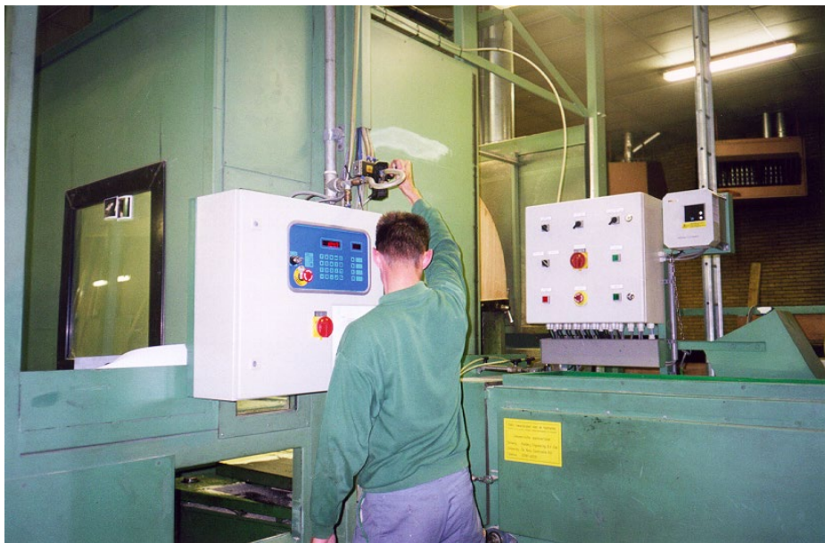
Operator initiating the opening of the bandsaw casing
