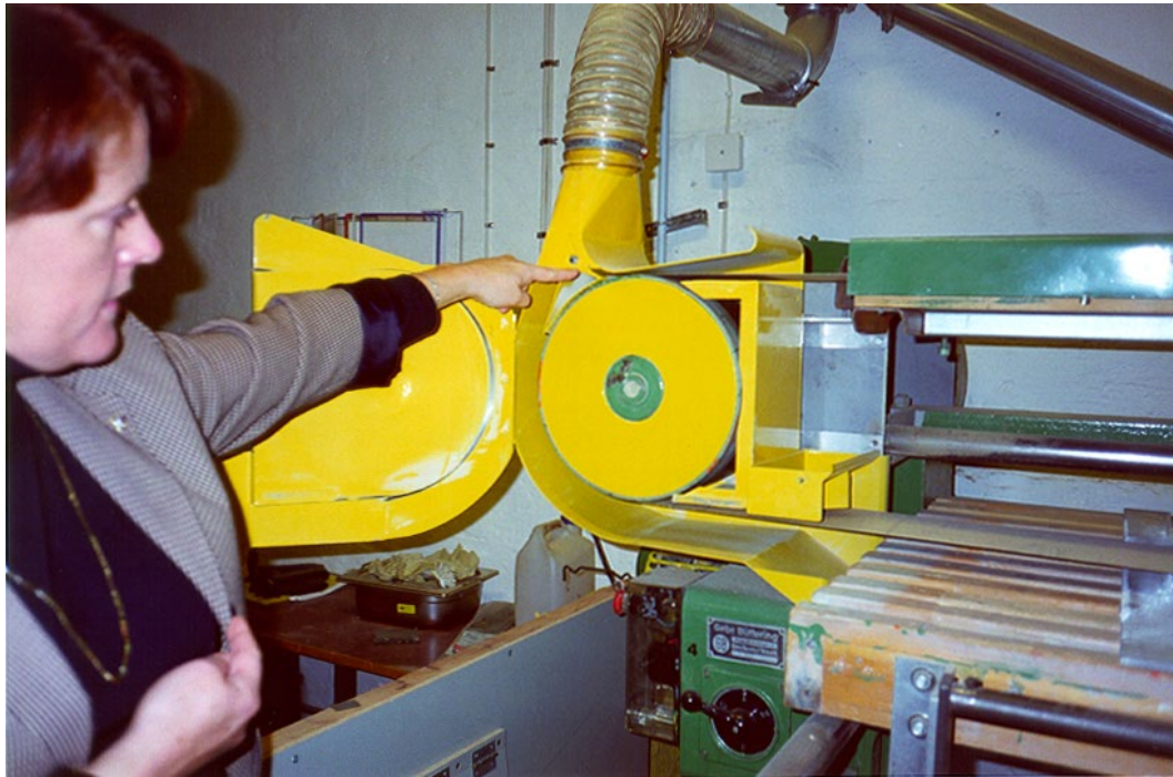
extraction unit on sanding belt - Tratek Jonkoping, Sweden
