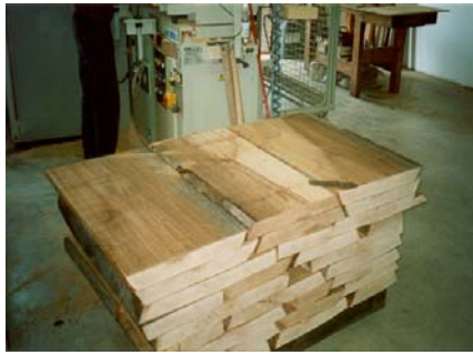
Slabs ready for componentry machining Pneumatic chair assembly line put together components in less than a minute. Chair legs balanced and squared.
