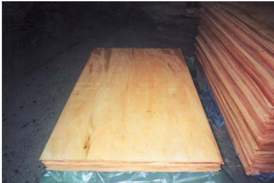
Plate 9 : Rotary peeled E. grandis veneers
