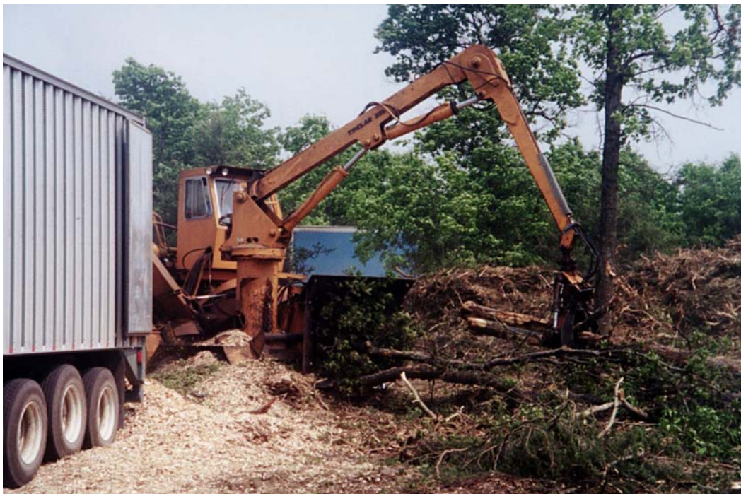
Figure 44 Trelan 23L disc chipper, chipping directly into a chip bin
