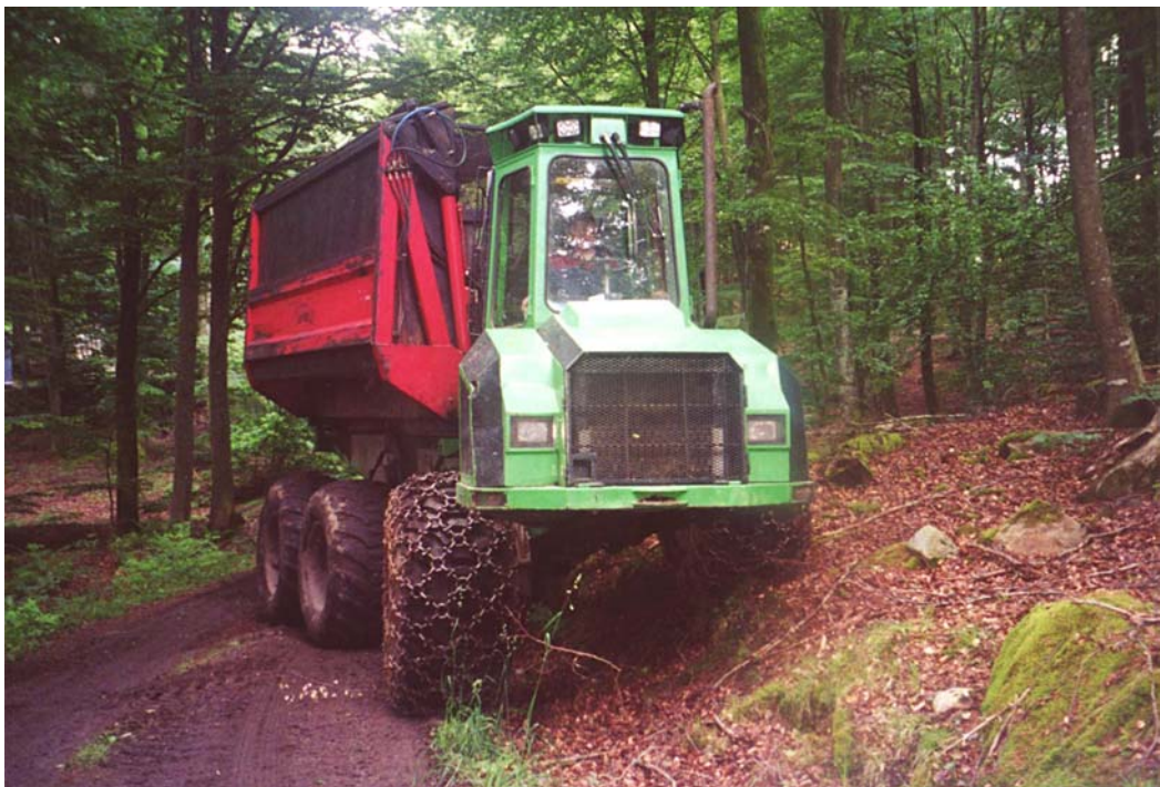
Figure 33 Demonstration of the capabilities of the self-levelling forwarder (bogies have a 130 cm travel range) (NB uphill wheels)
