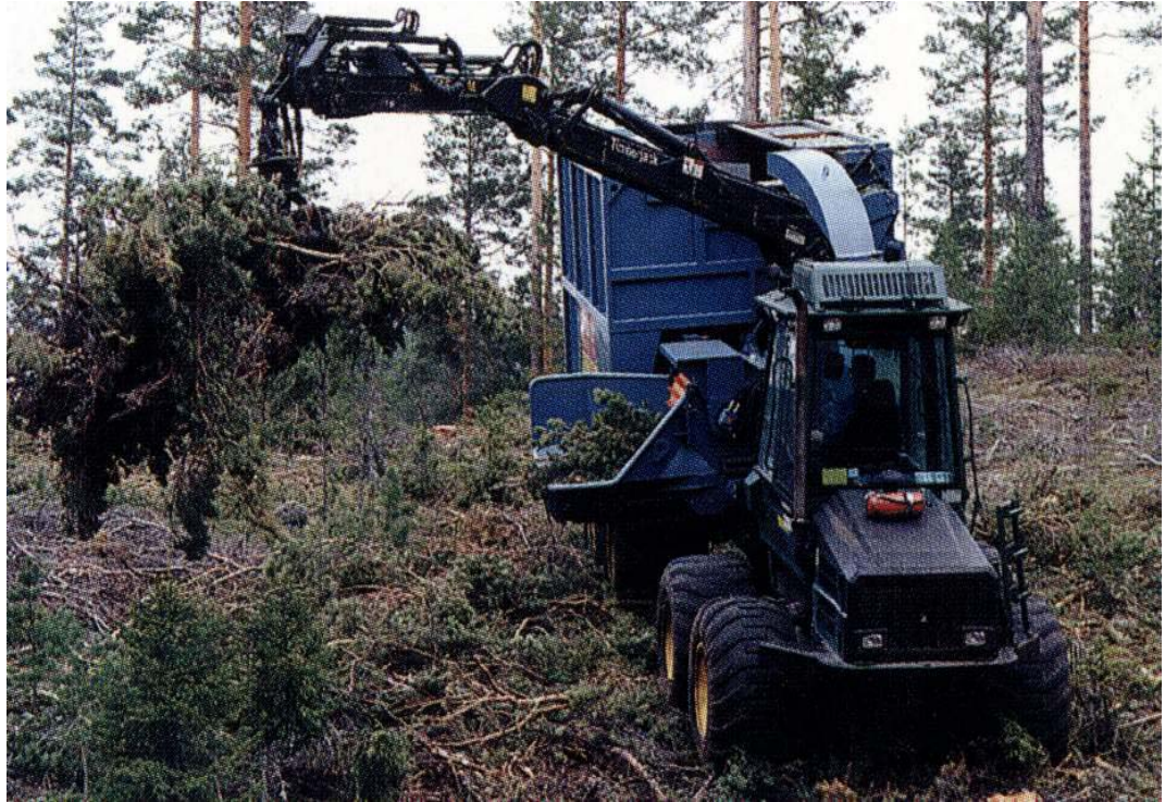
Figure 24 In-forest chipping using Bruks 804 CT model chipper
