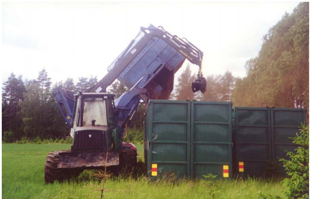
Figure 27 Bruks chipper unloading material into pre-positioned bins
