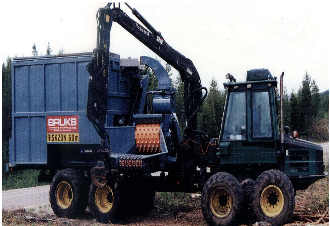
Figure 24 In-forest chipping using Bruks 804 CT model chipper
