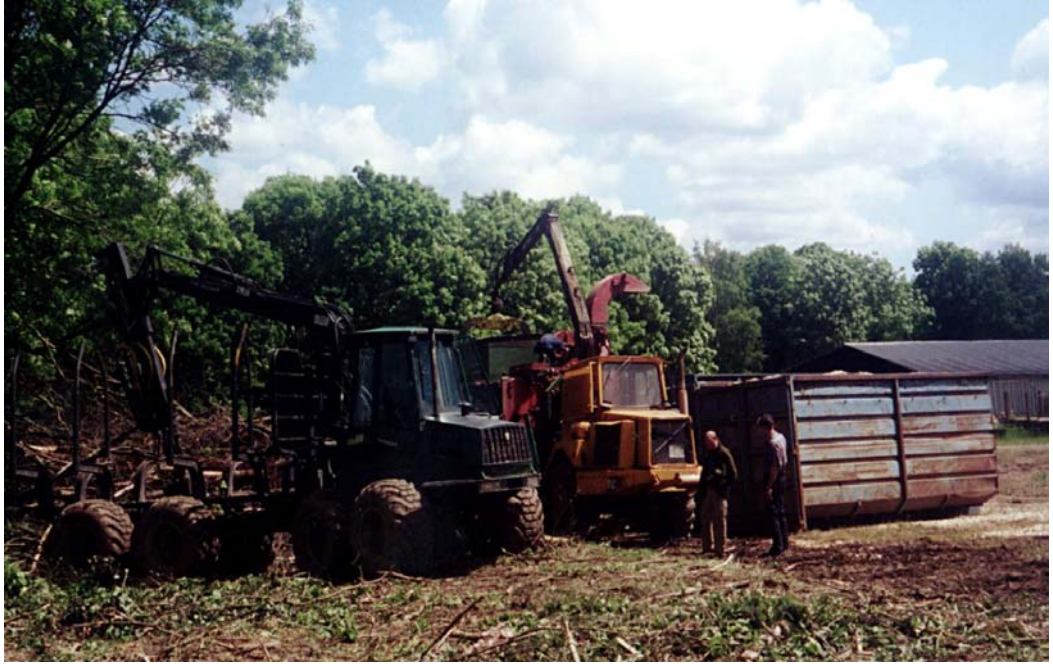
Figure 34 Roadside processing directly into chip bins using a remote controlled stationary chipper.
