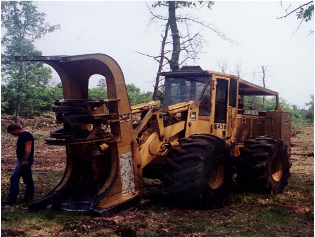
Figure 41 Feller-buncher (John Deere 643) fitted with a 'hot saw'
