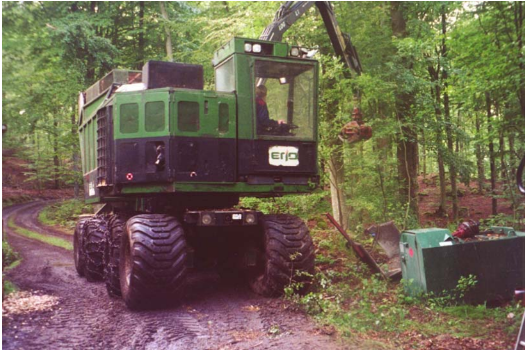
Figure 30 Purpose built chipper with 180° rotating cabin (mounted on a turntable) & rear storage bin
