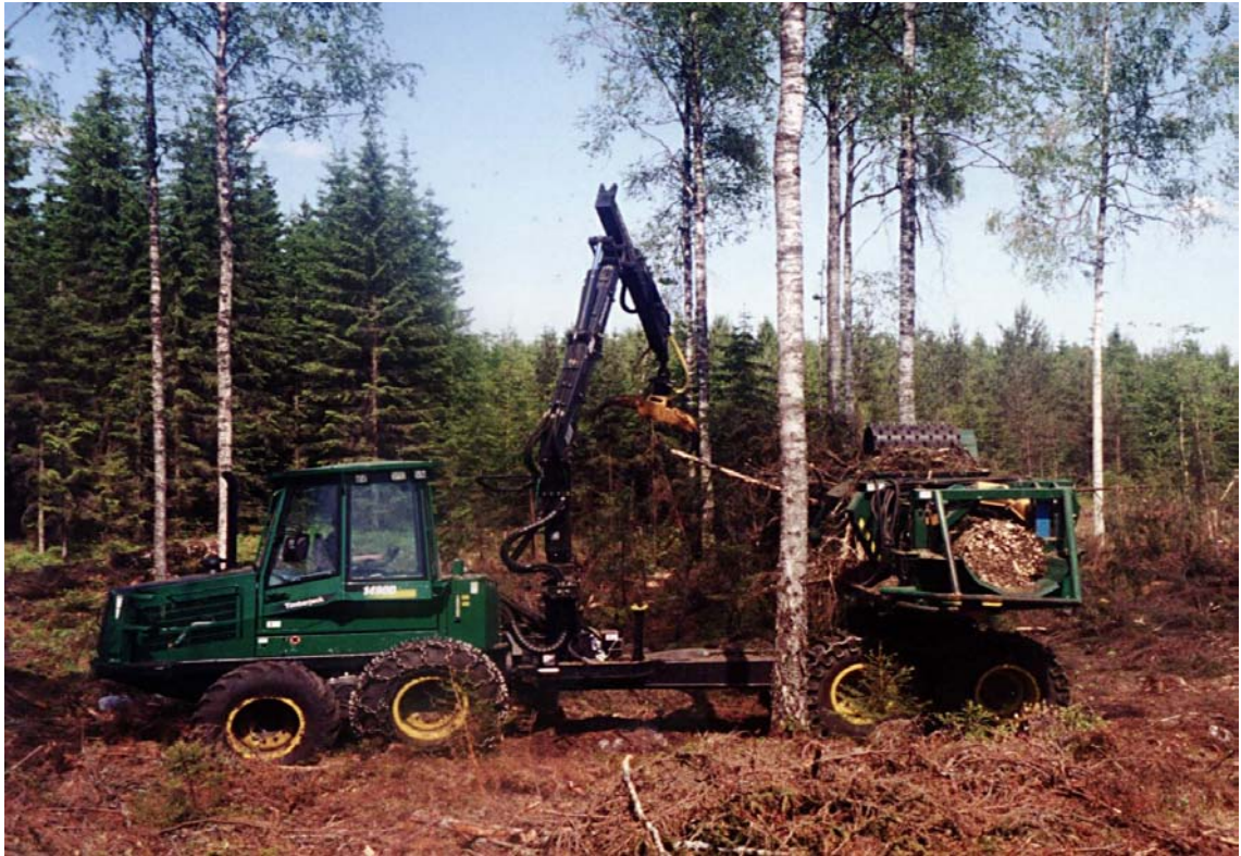
Figure 13 Timberjack Bundling System
