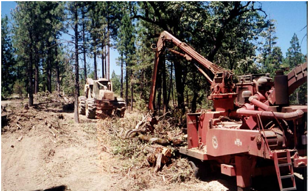
Figure 57 Whole-tree chipping of poor-form pine on private land near Redding.
