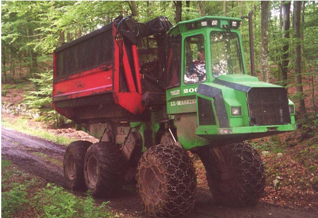
Figure 32 Purpose-built chip bin forwarder (25 m 3 capacity) with self-levelling capability
