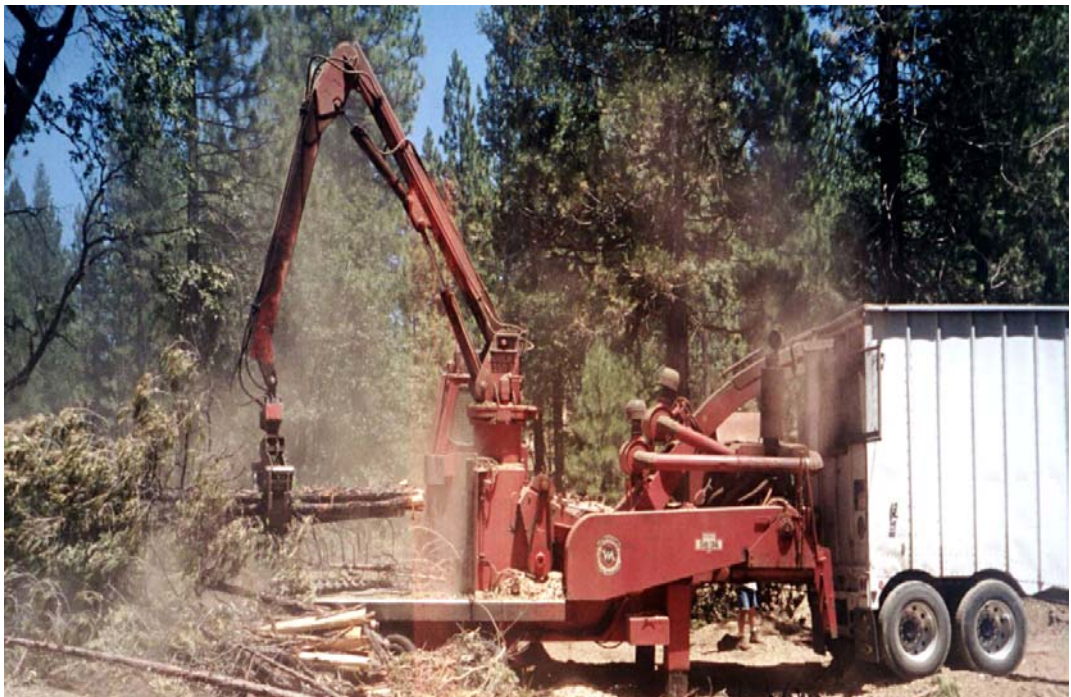
Figure 59 Whole tree chips are blown directly into chip bin for transport to Anderson Power Station.
