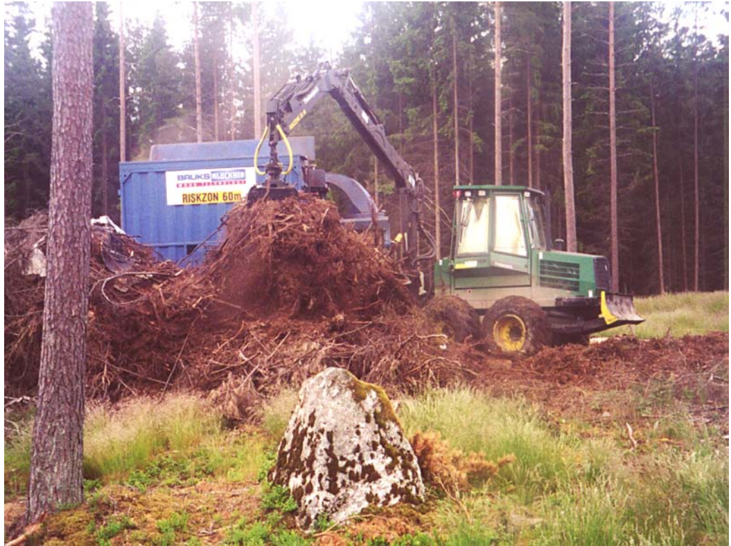
Figure 26 In-forest chipping of seasoned logging residue (Bruks 804 CT mounted on Timberjack 1410B forwarder)
