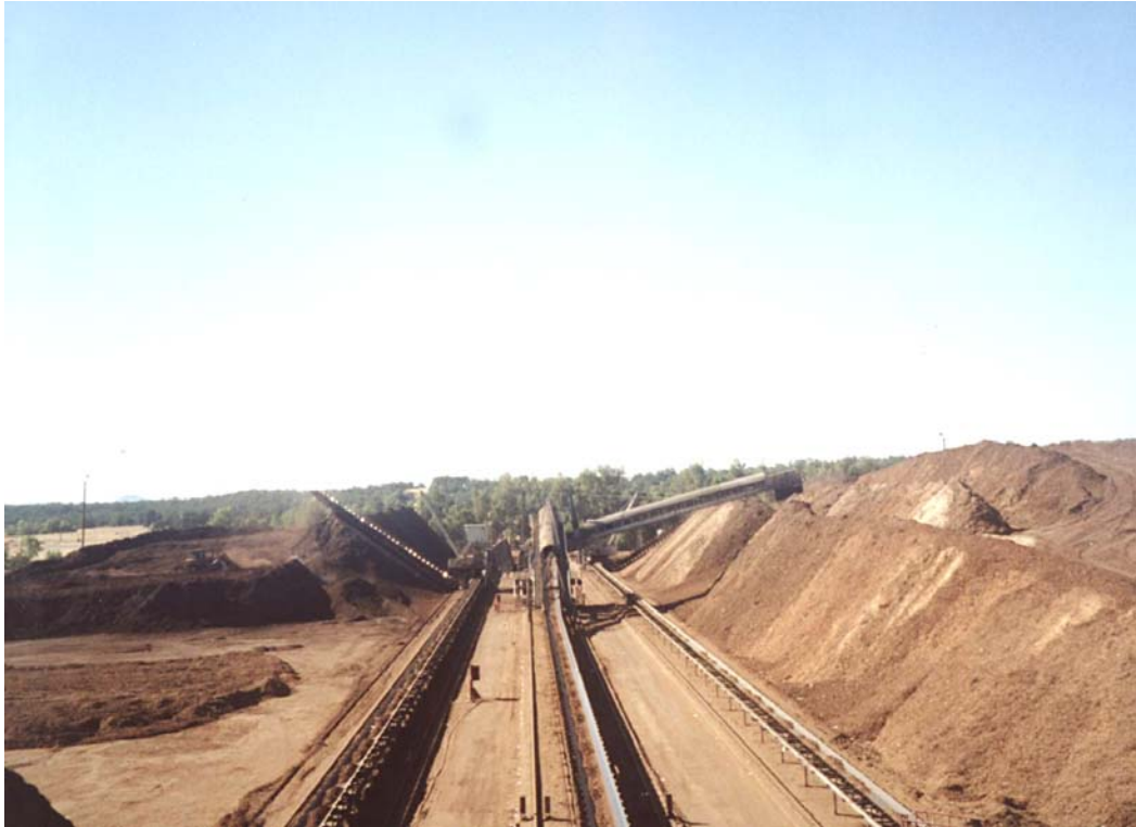
Figure 55 View of the Anderson plant's fuel stockpile. Twin reclaim lines continuously overfeed the plant's 3 boilers
