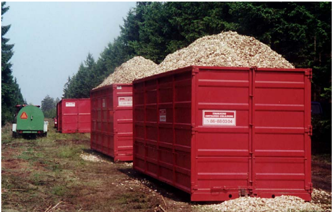
Figure 39 Flat-bed containers awaiting collection (normal truck payload: 60 m 3 , configuration 3 x 20 m 3 bins)
