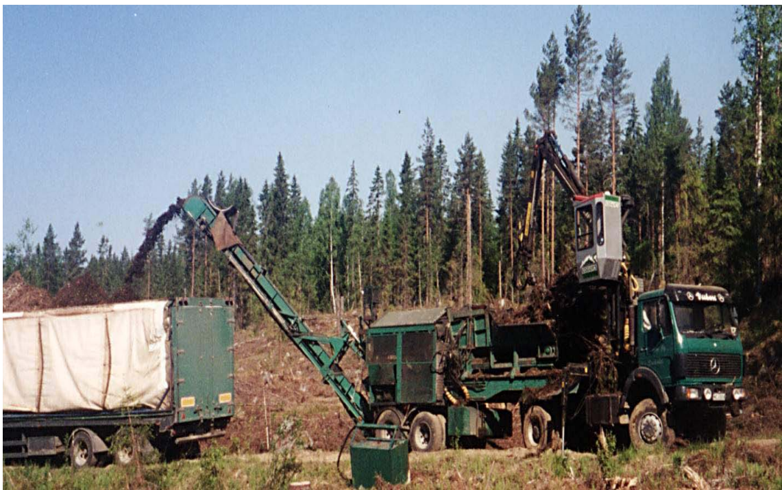
Figure 10 Roadside processing using a truck-mounted drum chipper
