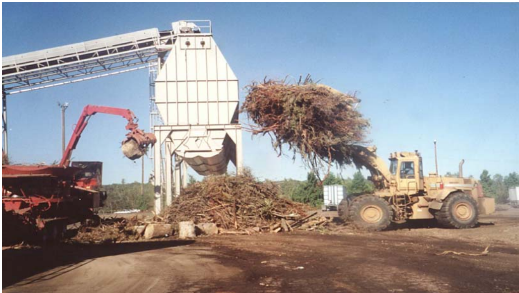
Figure 61 Loader feeding tub grinder. Material is fed onto secondary reclaim chain for delivery to the main stockpile.
