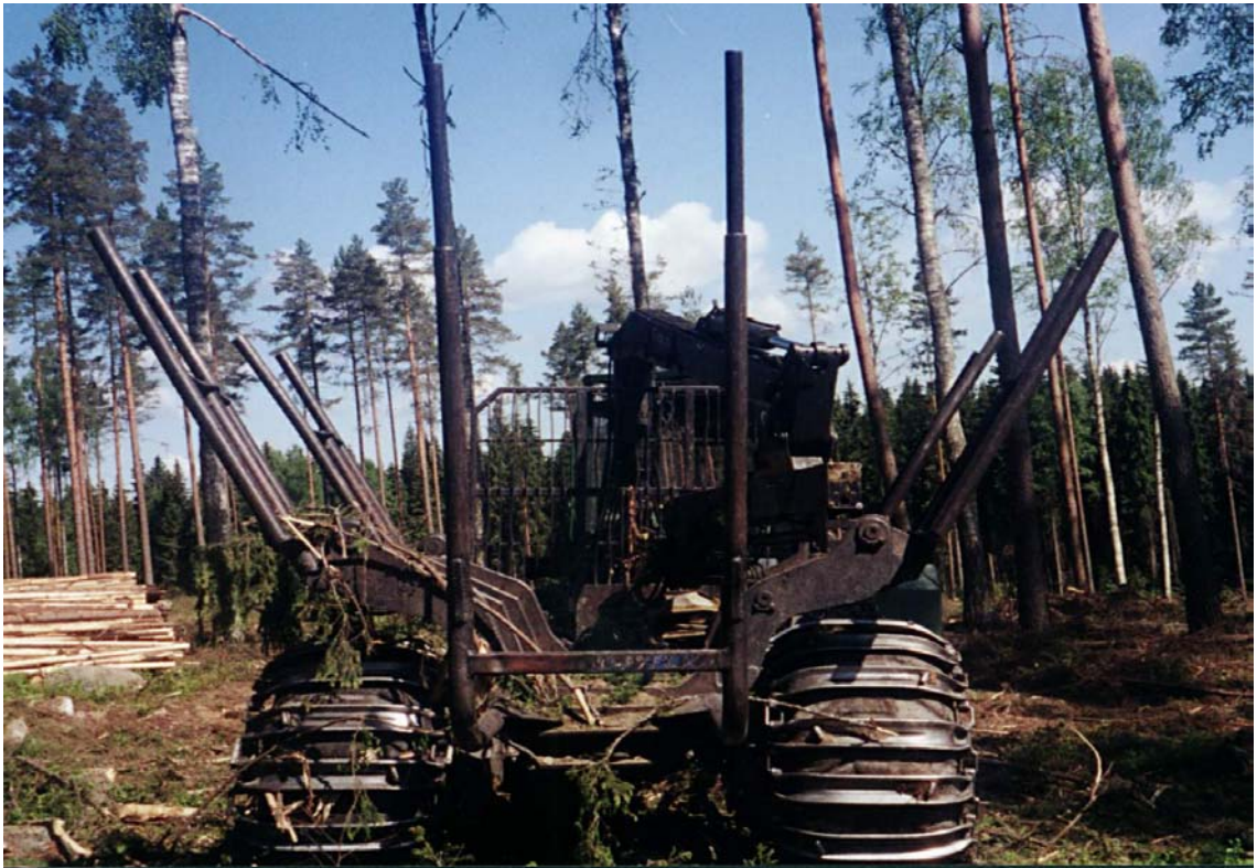
Figure 8 Modified forwarder (for greater payloads) used for logging residue extraction
