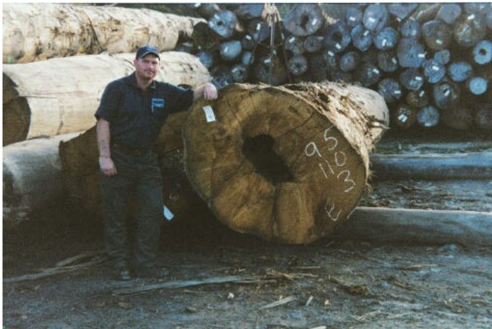
Figure 17. Noel Hall with a large E. muelleriana log exhibiting pipe.
