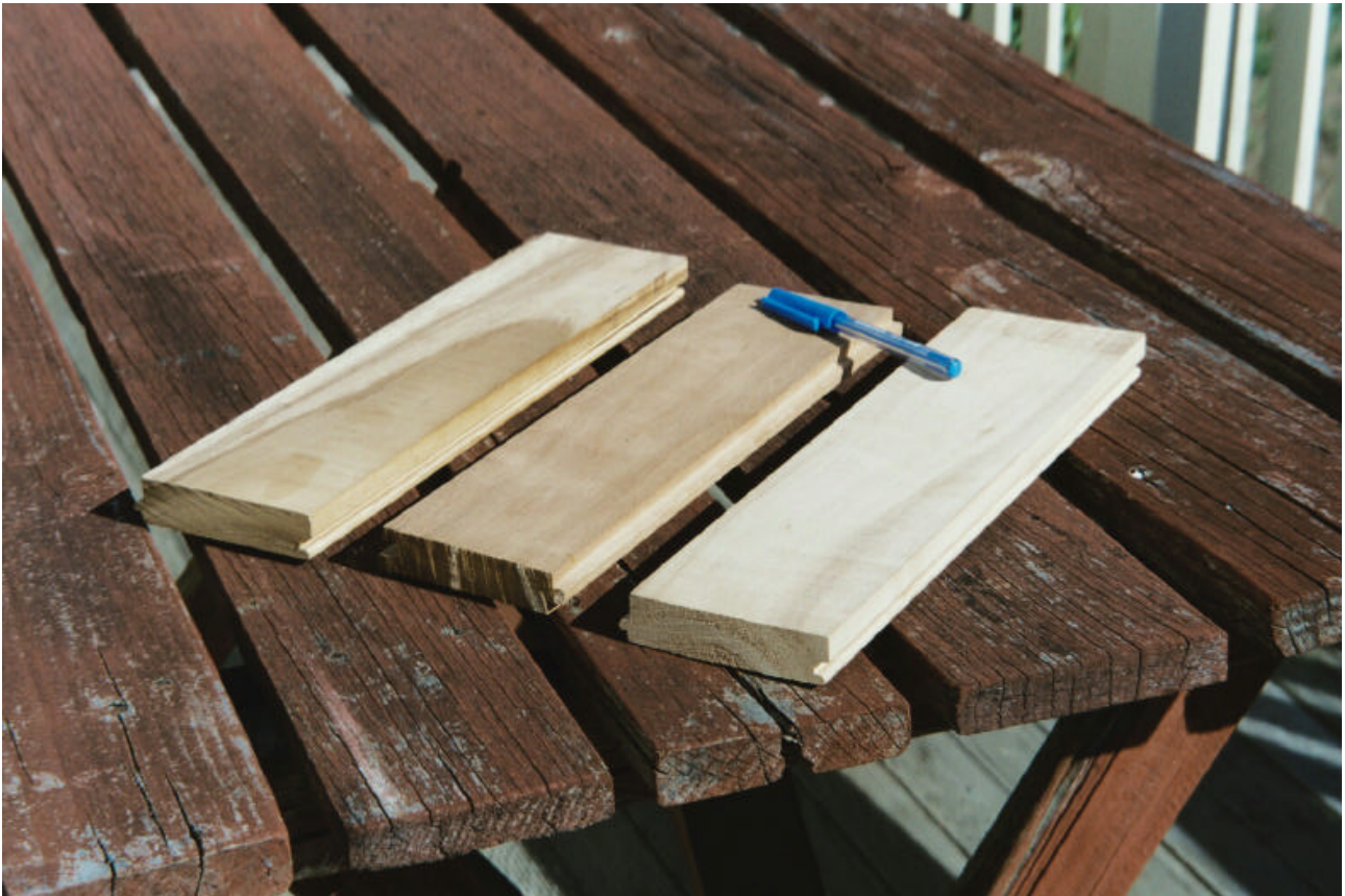
Figure 10. Backsawn boards (left and right) sawn from a 10-year-old E. muelleriana tree. The middle board is from native forest near Eden, Vic.
