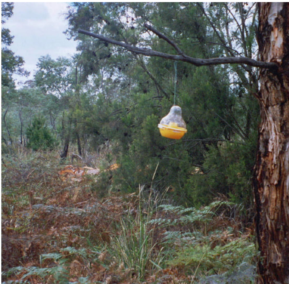
Figure 5: Dome trap used for vespid wasp capture.
