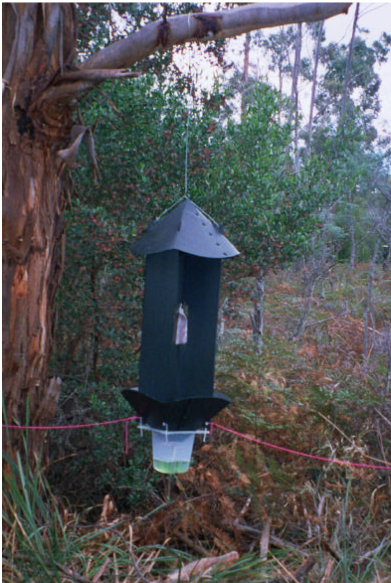
Figure 2: Intercept panel trap used for larger woodborers..
