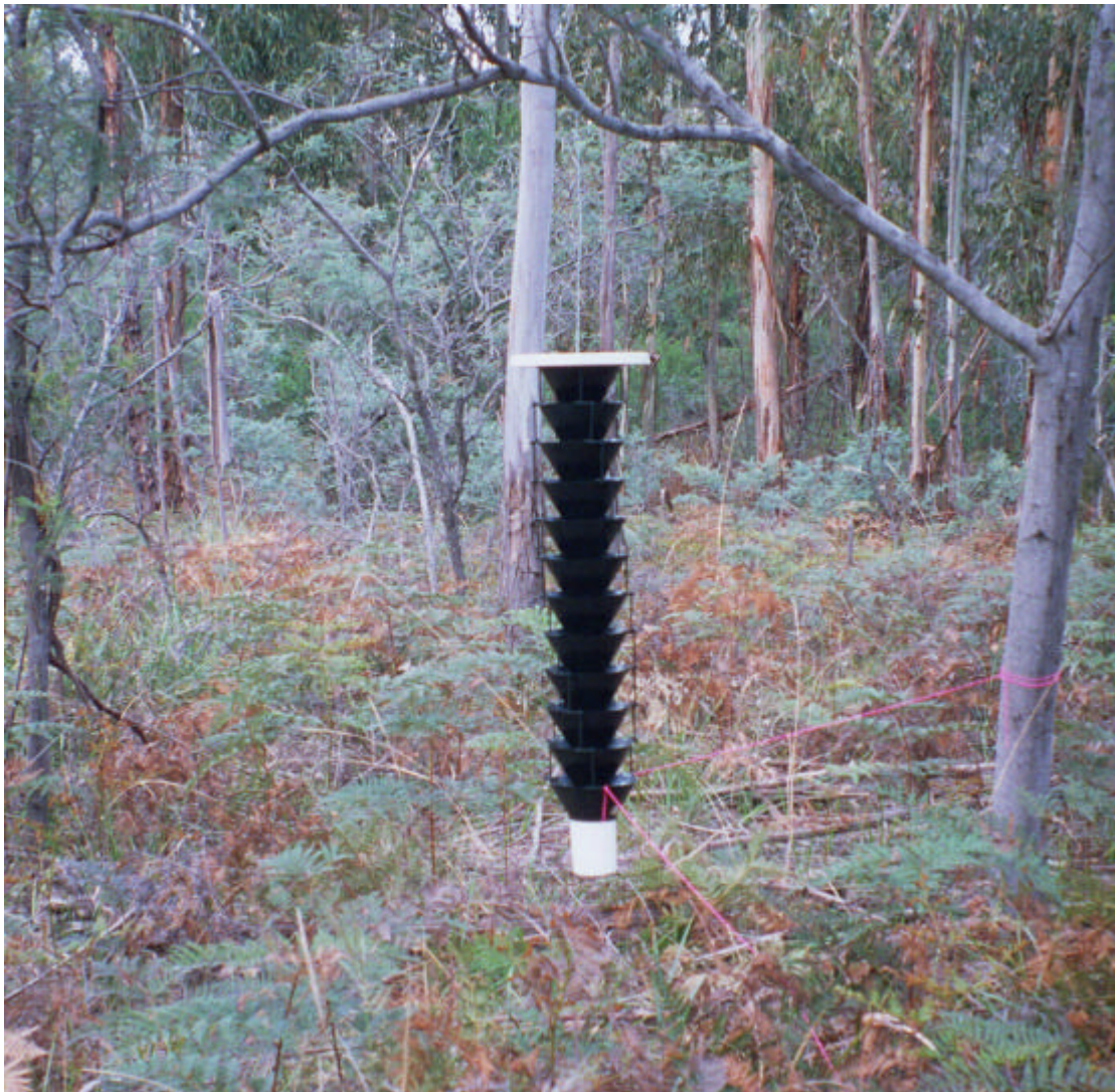
Figure 1: Lindgren 12-funnel trap uses for scolytids and platypodid beetles.
