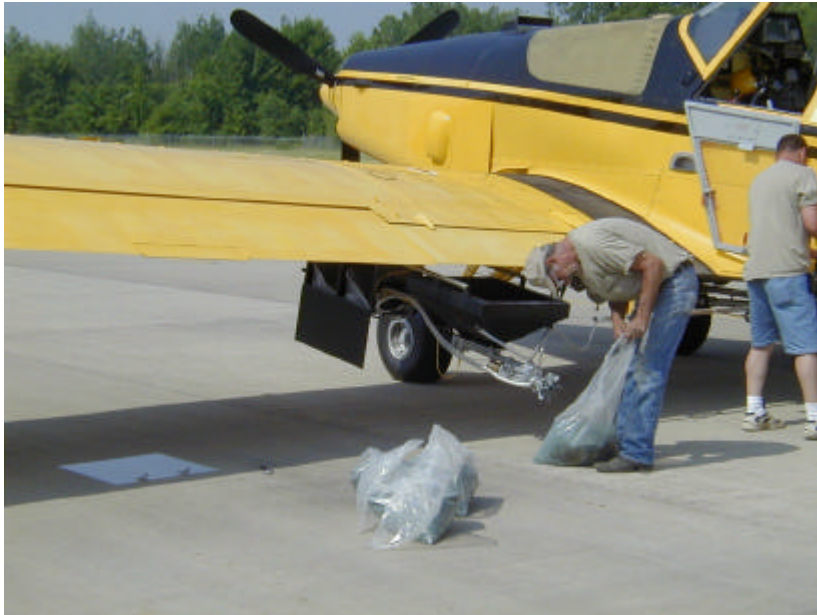
Figure11: Loading pheromone flakes into hopper beneath wing.
