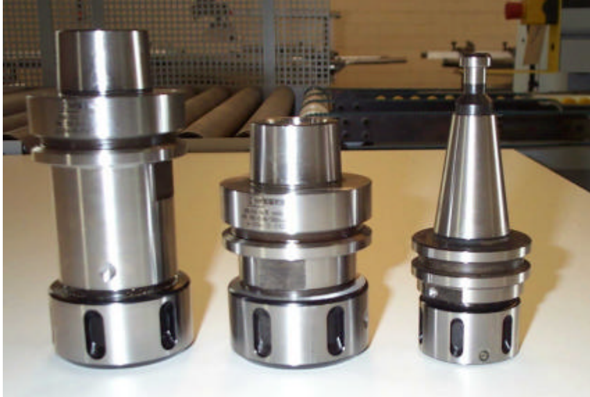
Figure 14 CNC tool holders left to right. Long HSK, Short HSK, SK (ISO30)
