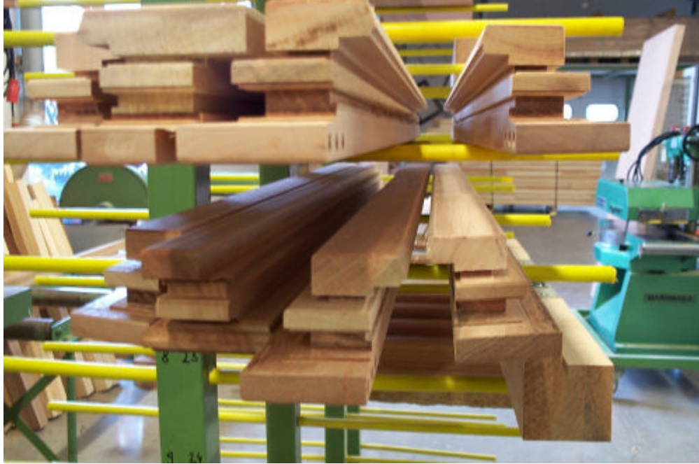
Figure 12 Complex window profiles produced with CNC at Nestle Fenster.
