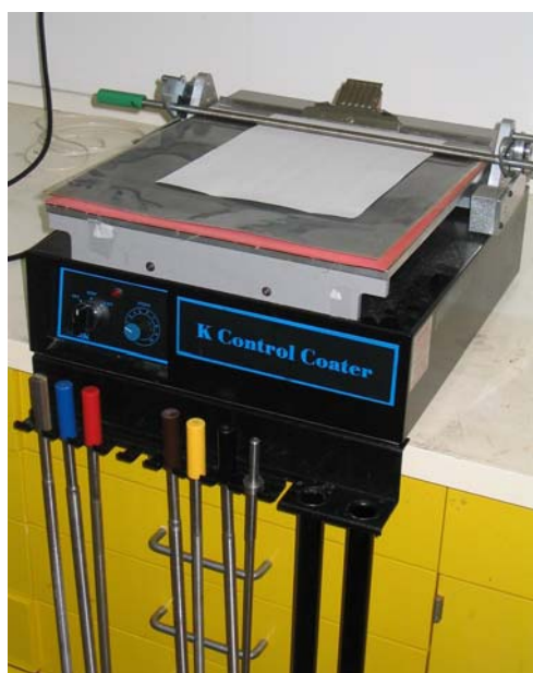
Figure 7- Drawdown coater for low speed coating of individual paper sheets.
