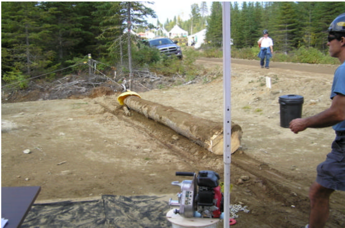
A 3.6 metre x 35 cm white pine log being pulled by portable winch. Also included in the photograph is a portable winch.
