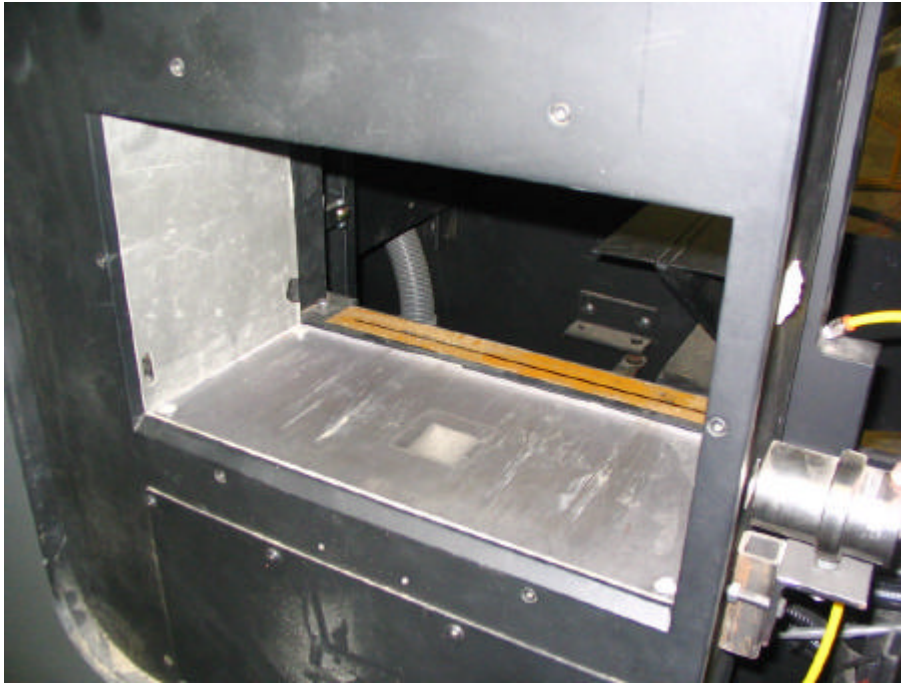
Fig. 39: LHG Microwave receiver with x-ray detector (thin strip) mounted behind (Coe Newnes/McGehee LHG laboratory)
