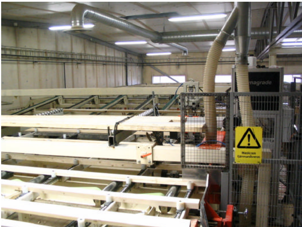
Fig. 15: Dynagrade Dynalyse – main unit obstructed by guard (Derome sawmill)
