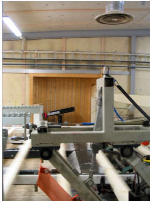
Fig. 17: Laser unit at far end – measuring board length (Derome sawmill)
