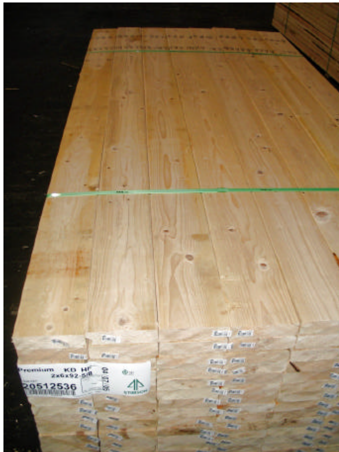
Fig. 31: Hemlock stud material graded by the D*TEC BioScan (Stimson Lumber Company)
