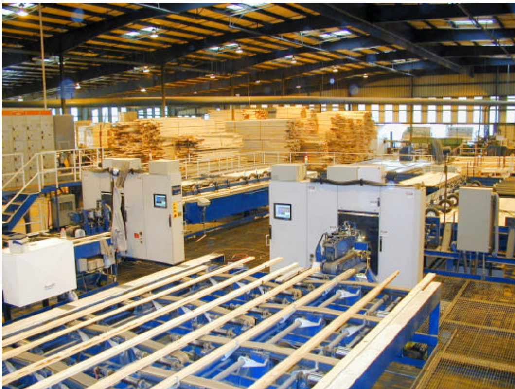
Fig. 41: ChopScans grading for finger-joint feedstock (Sierra Pacific, Red Bluff – courtesy Lucidyne Technologies)
