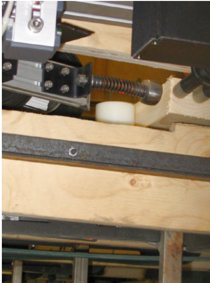
Fig. 16: Detail of spring-loaded hammer & microphones (Derome sawmill)
