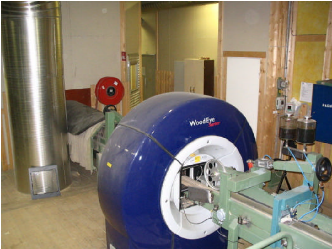
Fig. 35: Woodeye Sorter close-coupled to planer (Stora Enso Kopparfors mill)
