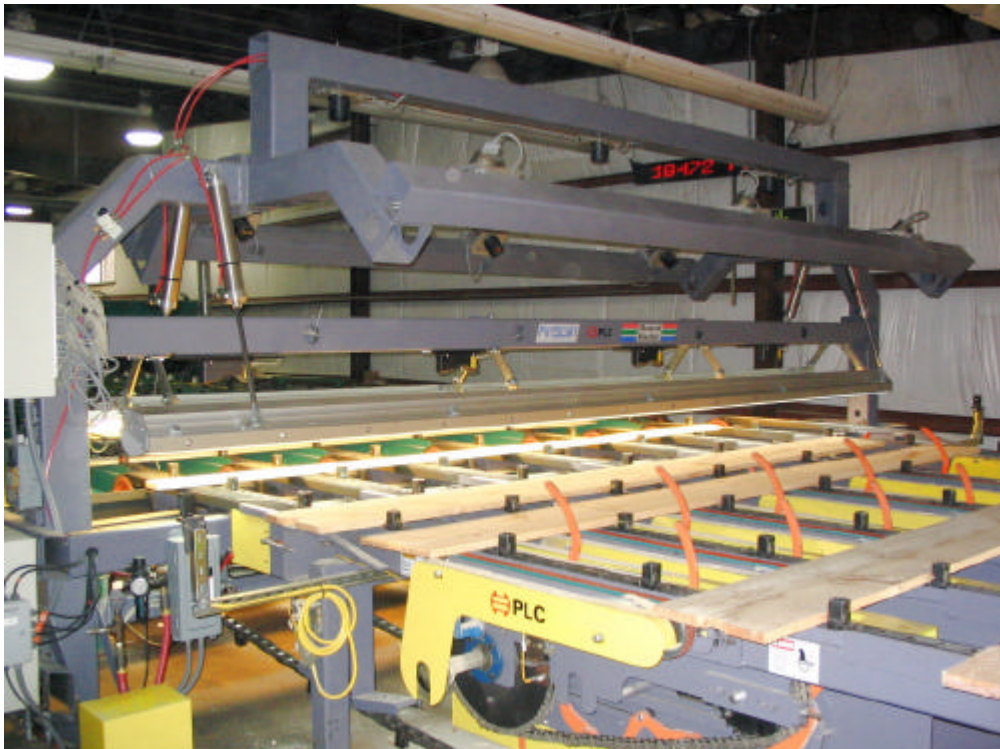
Fig. 33: Scanner Frame 2 & board turner (Durgin & Crowell)
