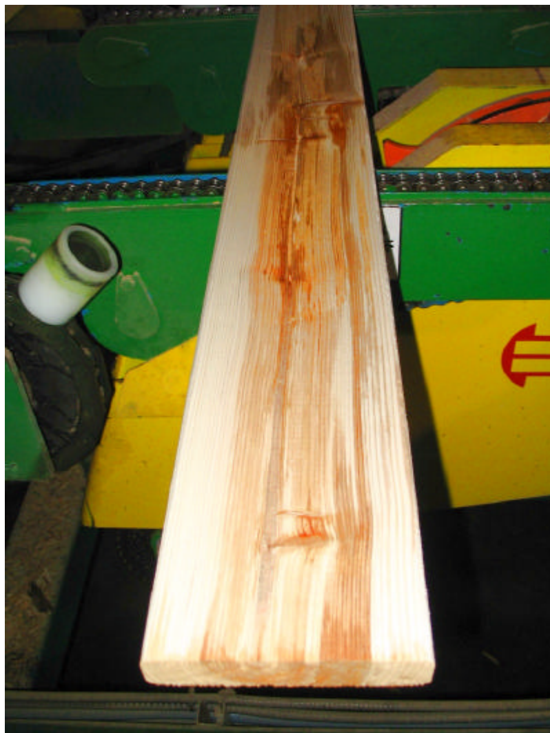
Fig. 25: Rot on board ends – issue for UV reader
