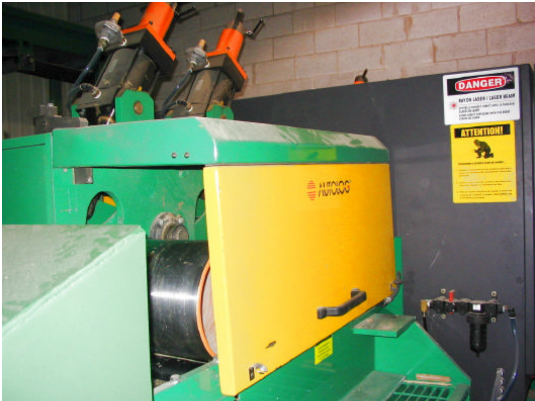
Fig. 22: Autolog LPO – outfeed press rollers & pneumatics for size change (Claude Forget Inc mill)
