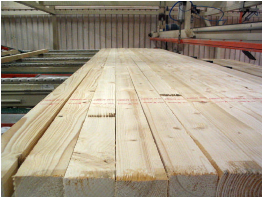
Fig. 18: Spruce graded by the Dynagrade at Derome sawmill – note small knot size
