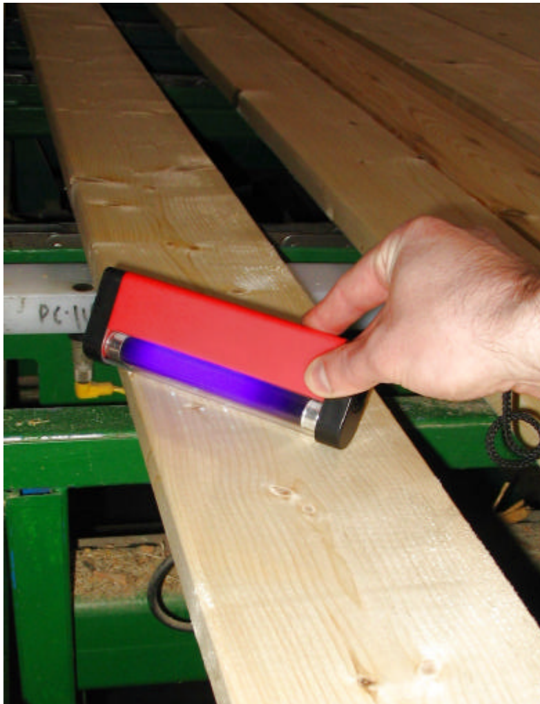
Fig. 21: Illumination of UV binary code (Claude Forget Inc mill)
