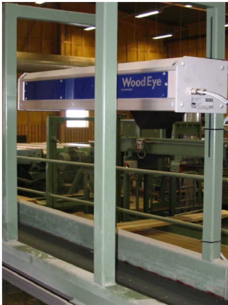
Fig. 37: Downstream warp sensor (Stora Enso Kopparfors mill)
