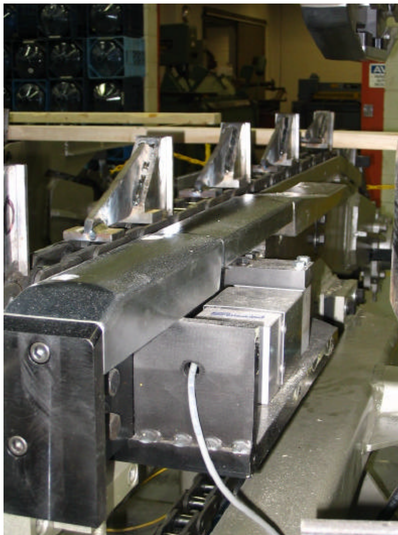
Fig. 13: Underside shoe with integral load cell for measuring resistance to deflection (CRIQ laboratory)
