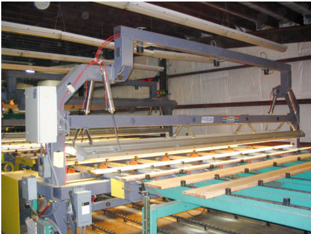
Fig. 32: FinScan Boardmaster NT – Scanner Frame 1 (Durgin & Crowell Lumber mill)
