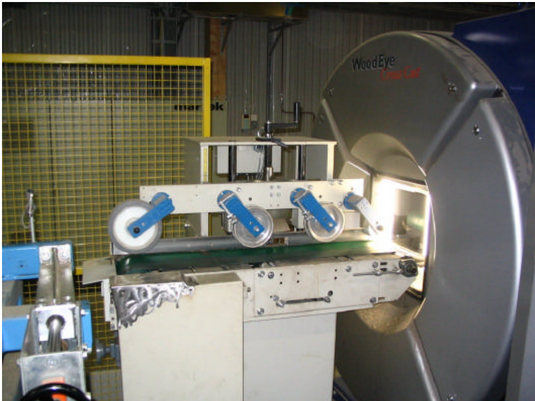
Fig. 36: WoodEye CrossCut – infeed & scanning field (Stora Enso Ala mill)
