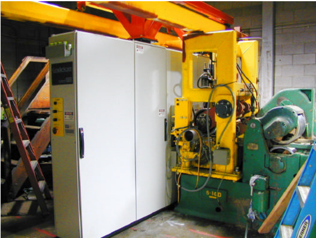
Fig. 40: Lucidyne GradeScan close-coupled to planer (Seneca, Eugene – courtesy Lucidyne Technologies)
