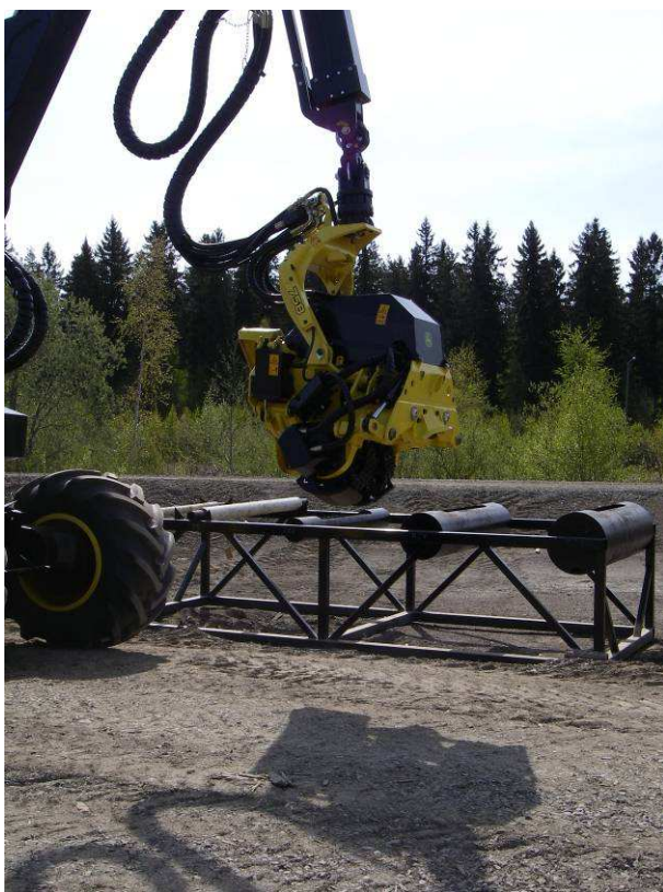
Figure 17 – Calibration Using Metal Pipes at John Deere Factory
