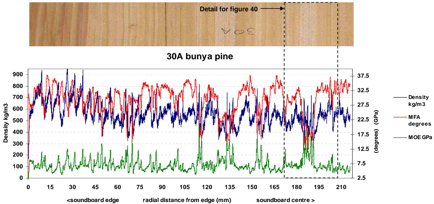
Figure 39. Plate 30 (guitar two) Mean: density 560 kg/m<sup>3</sup> - MOE 7 GPa- MFA 30 ° - along grain sound velocity 3773 m/s
