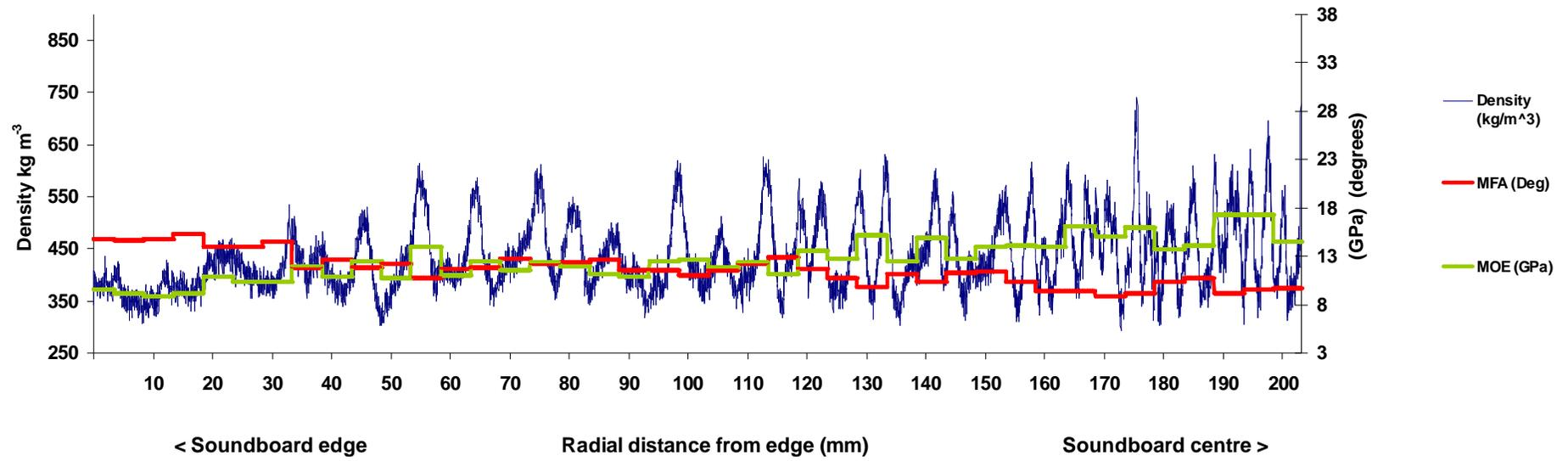
**Appendix 6** Silviscan-derived wood properties and corresponding strip from soundboard half
