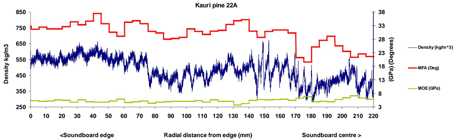
**Appendix 8** Silviscan-derived wood properties and corresponding strip from soundboard half
