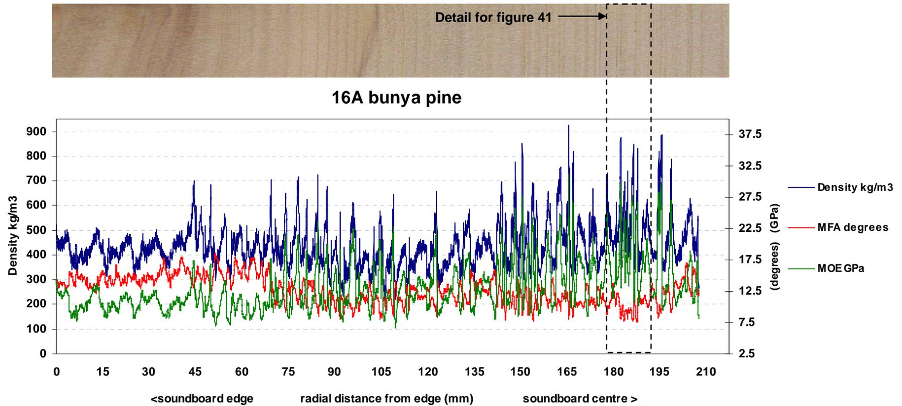
Figure 38 Plate 16 (guitar four) Mean: density 440 kg/m<sup>3</sup> - MOE 12.7 GPa - MFA 13° - along grain sound velocity 5674 m/sec.
