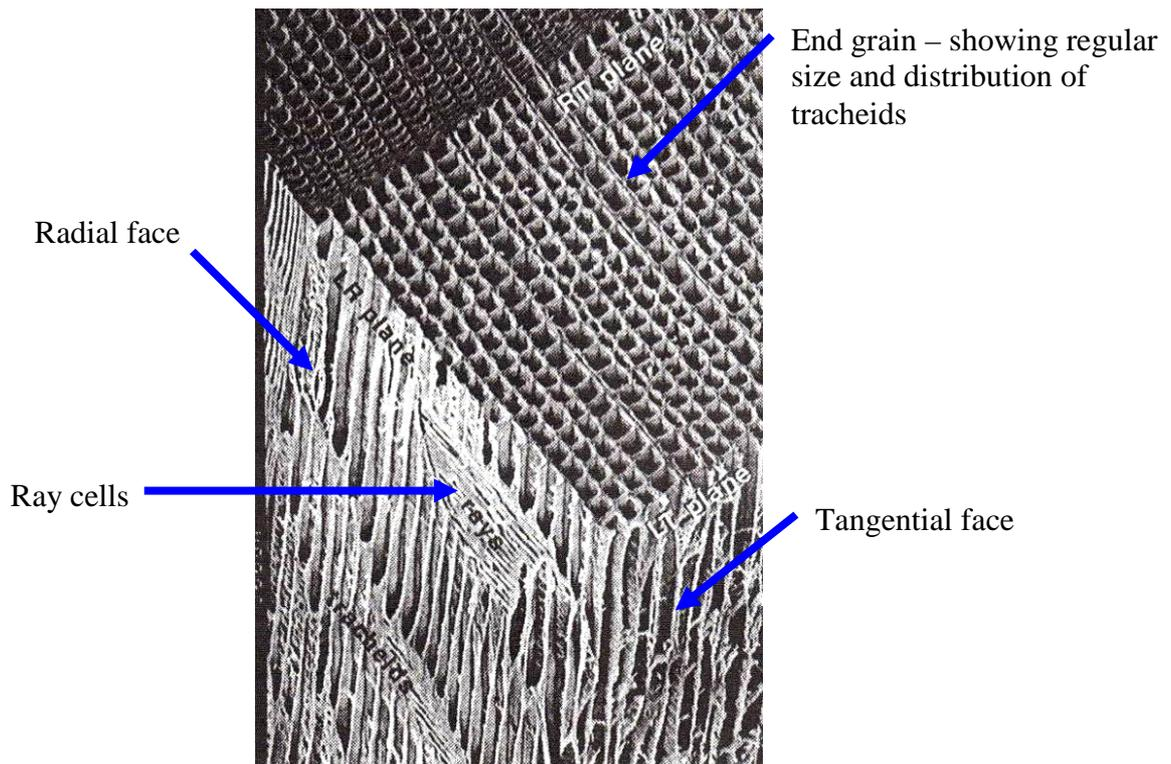
Figure 34. Scanning electron micrograph (SEM) of resonance spruce (photo courtesy of Bucur 2006)
