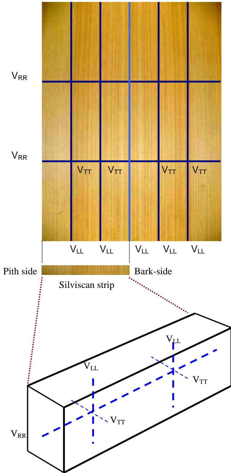
Figure 36 Measurement points on soundboard plates and Silviscan strips.
