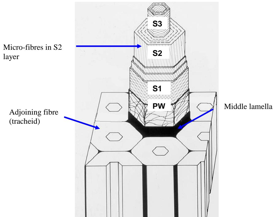
Figure 35 Representation of a fibre wall. PW indicating primary wall; showing the three cell wall layers. (source Downes *et al* 1997)
