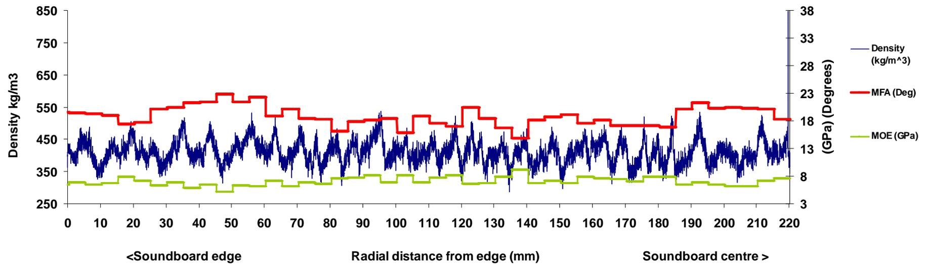
**Appendix 7** Silviscan-derived wood properties and corresponding strip from soundboard half
