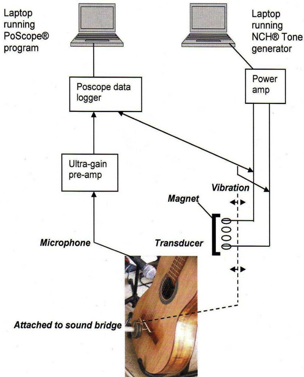
Figure 43. Schematic diagram of spectral analysis used in the objective evaluation of instruments (Equipment and methodology provided by Mr David Chin)
