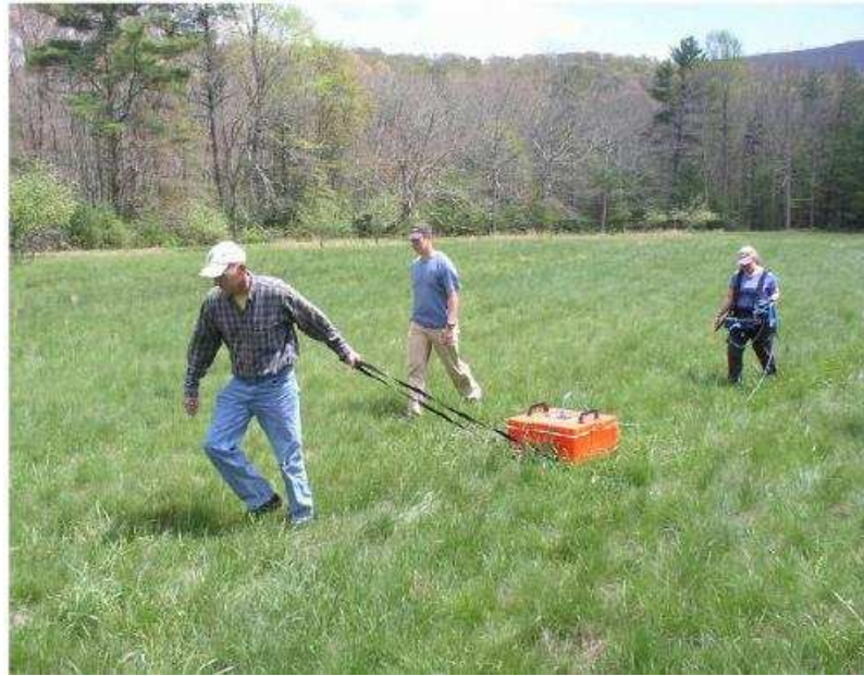
Figure 9. Ground-penetrating radar being pulled across the surface of the ground.
