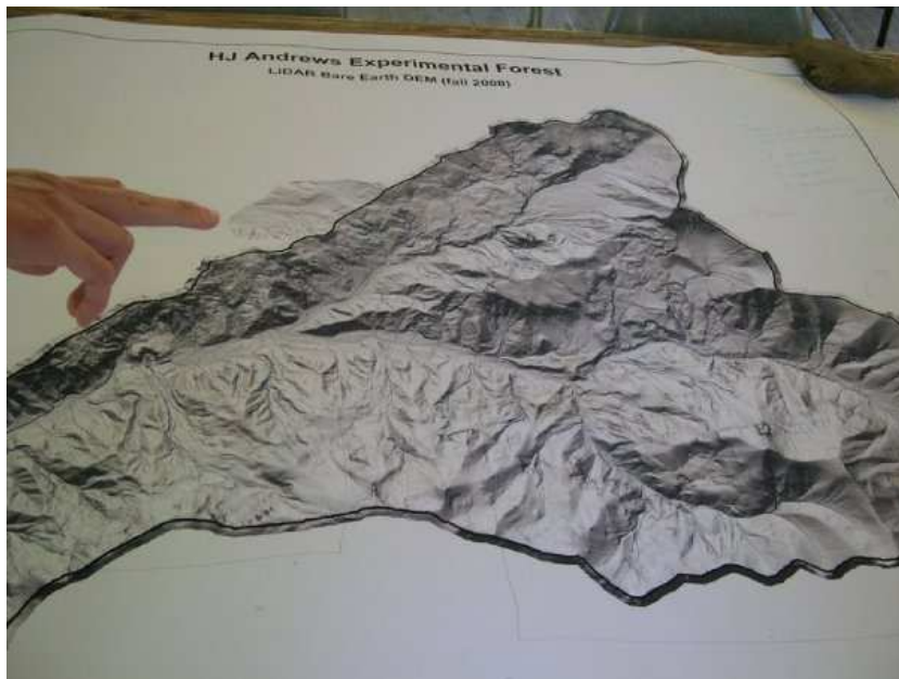
Figure 22. LiDAR Digital Elevation model used to help in identifying the locations of land slips
