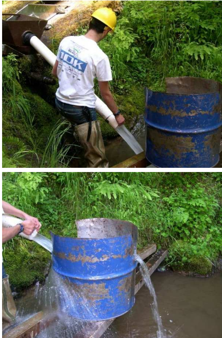
Figure 24. Stream volume being measured with calibrated 44 gallon drum
