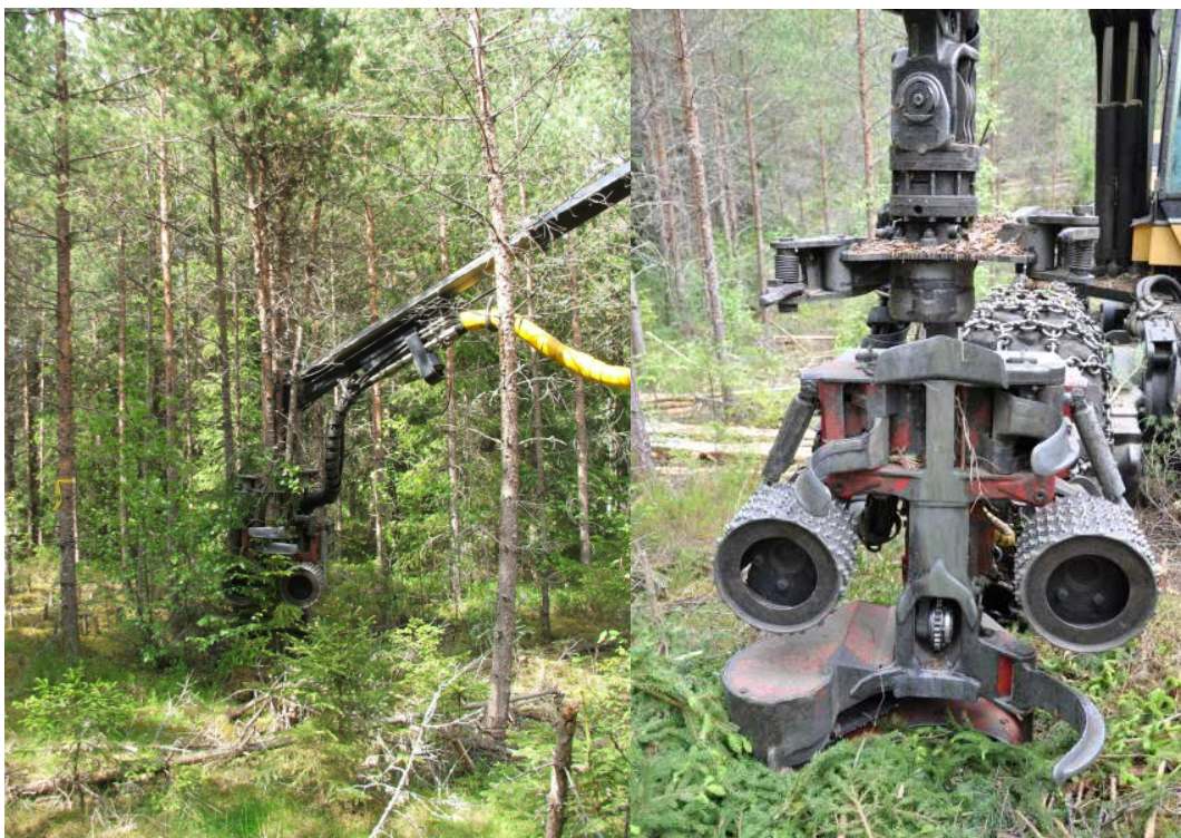
Figure 7. Multi Stem Harvester 560 C Ecolog Used in Thinning of Young Stands.
