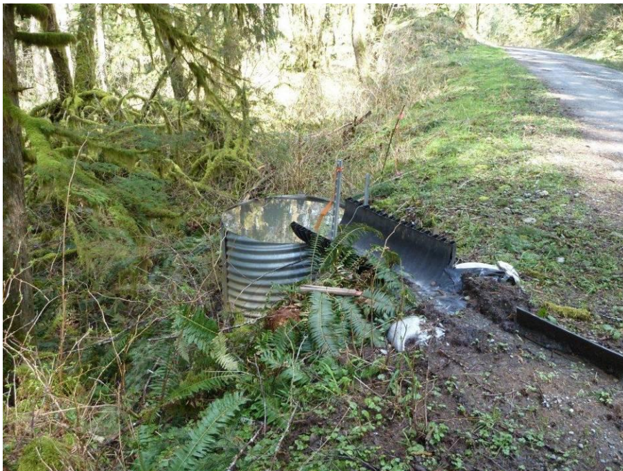
Figure 41. Road drainage is diverted into detention drums to allow measurement of the amount and type of sediment being produced by different road surfaces
