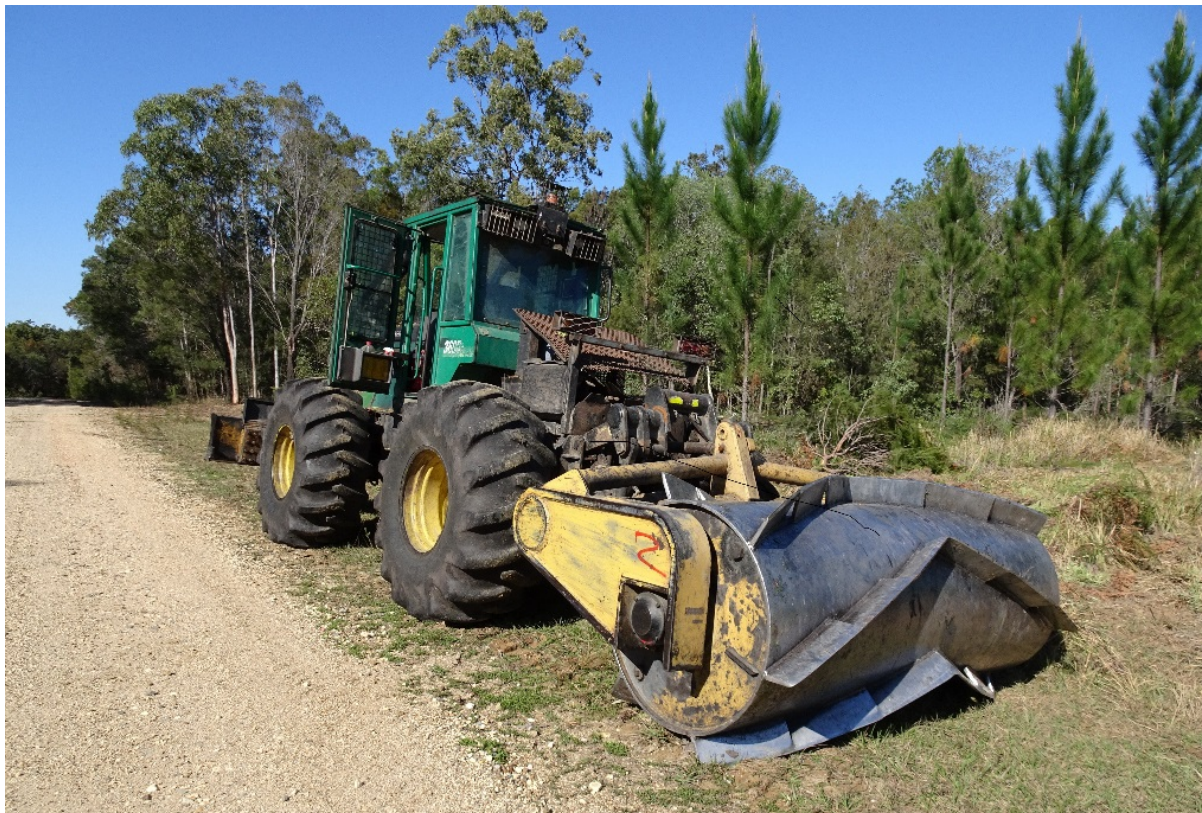
Figure 9: Chopper roller used as mechanical weed control inter row within their southern pine plantations, north of Gympie Queensland.
