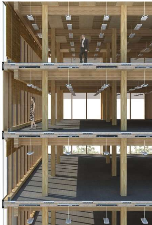
Figure. 5. Architect's impression of structure and services in the WIDC building (Source: Michael Green, http://mg-architecture.ca/work/wood-innovation-design-center/ )
