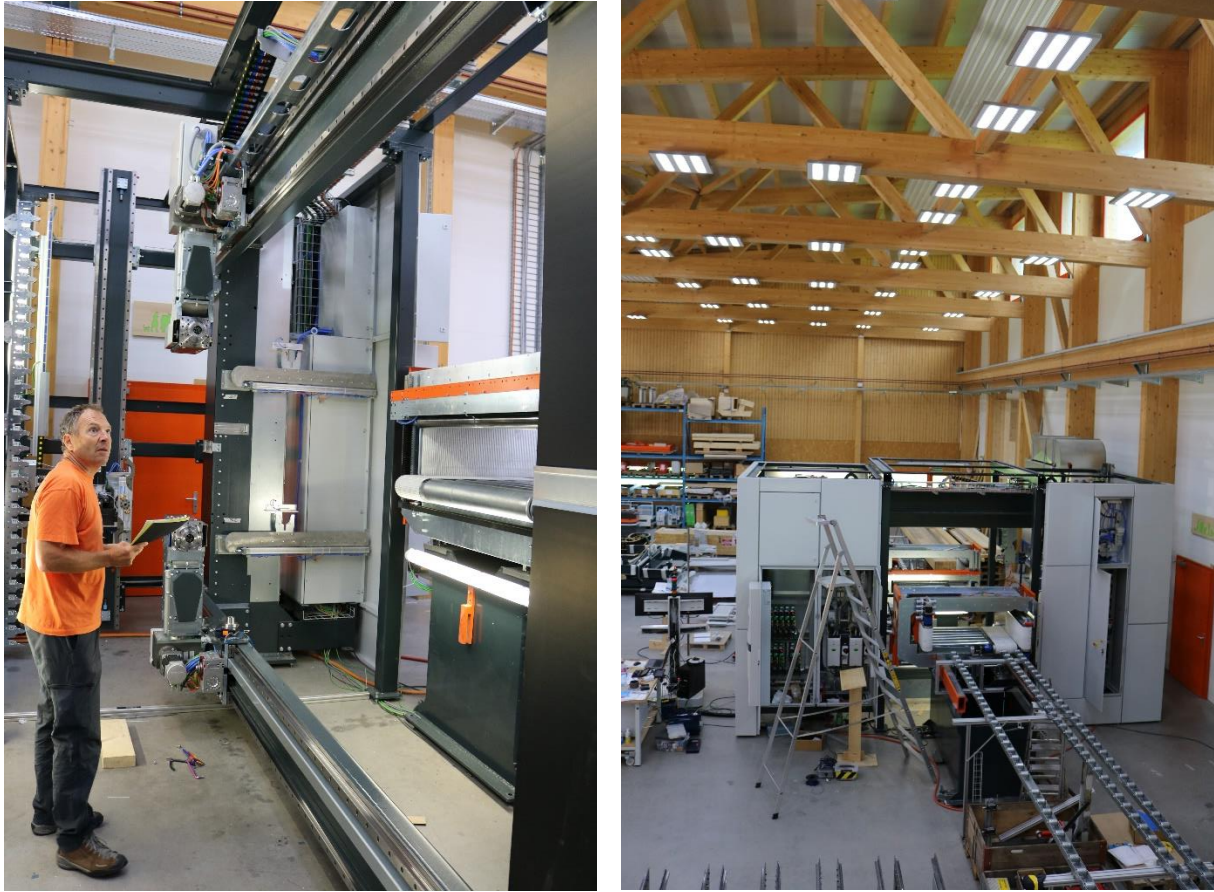
Figure 36. On the left, company founder and head designer Urs Steinmann standing inside the portal of a TW Agil Mill under construction, same machine on the right from outside the portal. Photos by Author
