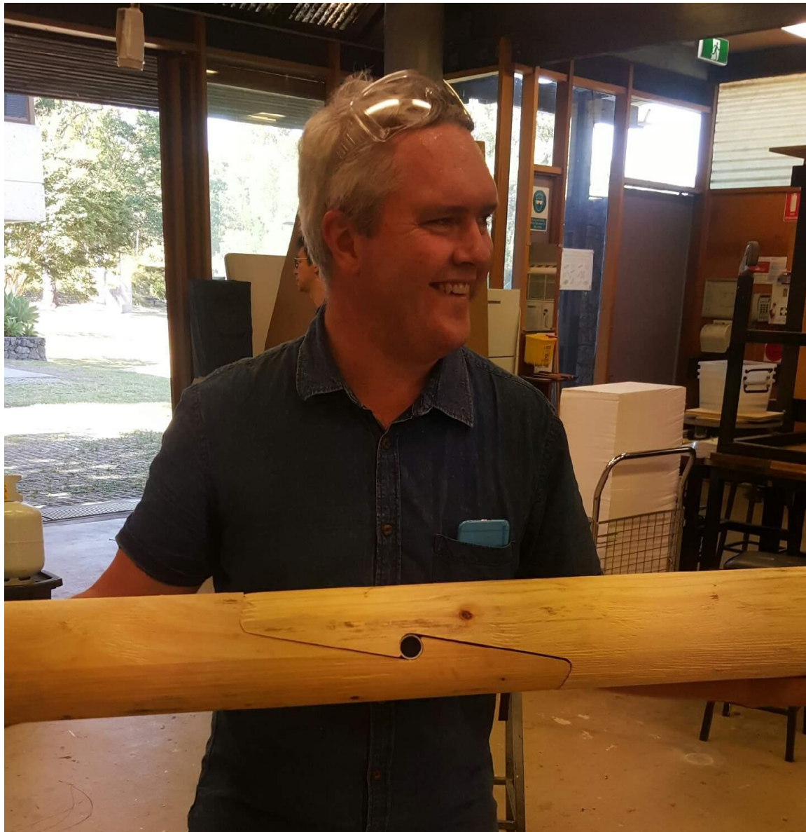
Figure 42. Author with the completed prototype. With the insertion of the locking pin the joint becomes rigid. Note: in this example an aluminium tubing has been used for ease of removal for demonstration purposes. Photo by Author
