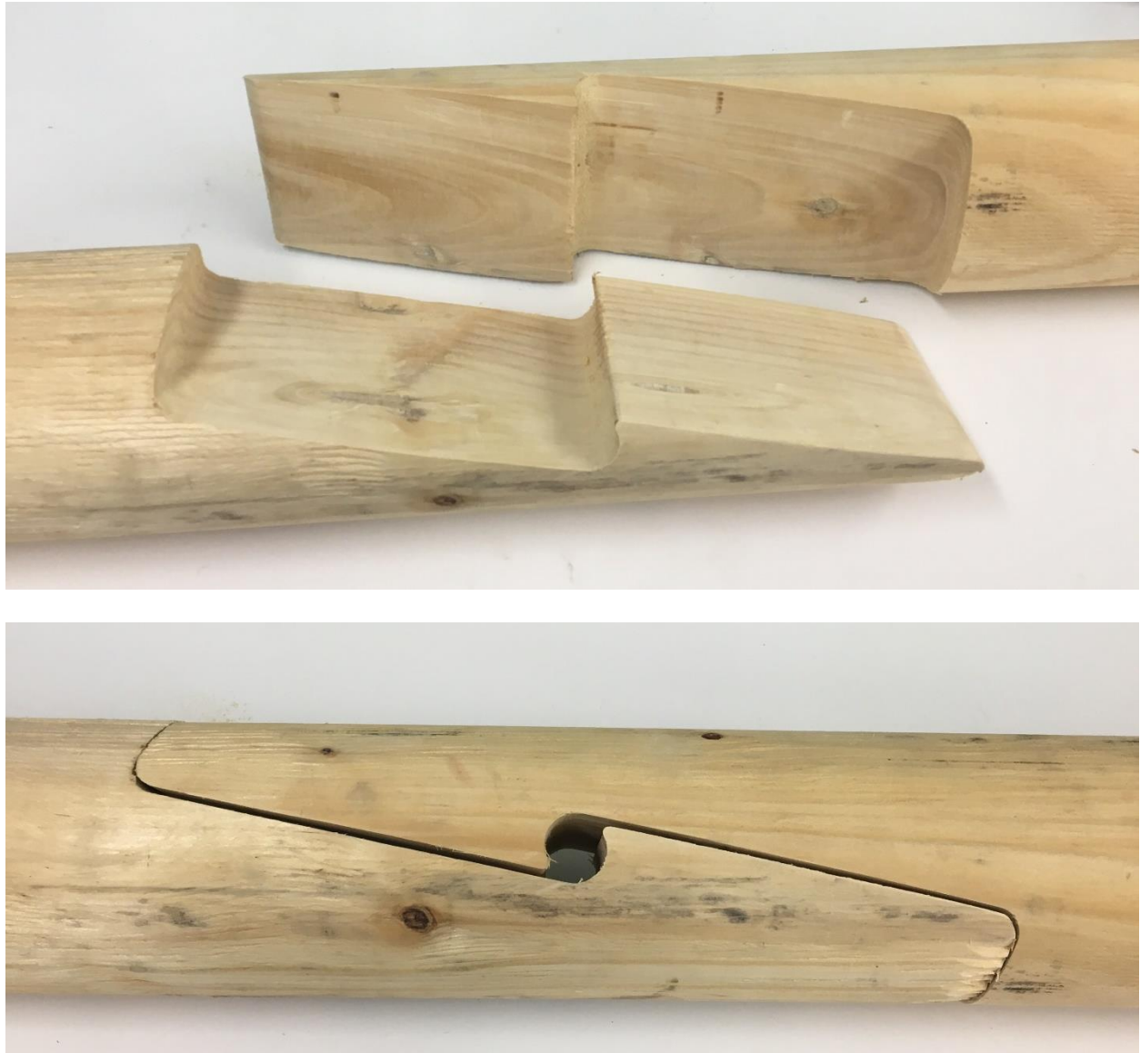
Figure 41. The locked hook scarf joint shown in both the open and interlocked configuration. Photo by Author.
