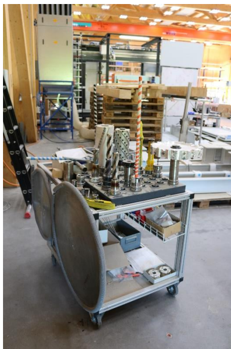
Figure 37. A selection of the tools that the mill can use, ranging from small router bits to planing heads and saw blades. The mill has an automatic tool changing station inside the portal. Photo by Author
