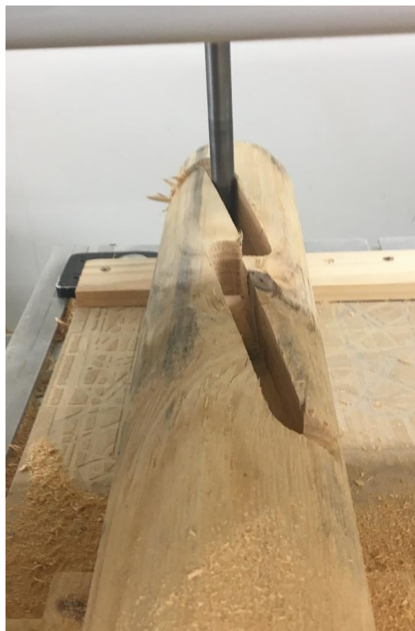
Figure 40. The geometry of the joint was coordinated with the machining constraints of the CNC router Photo by Author
