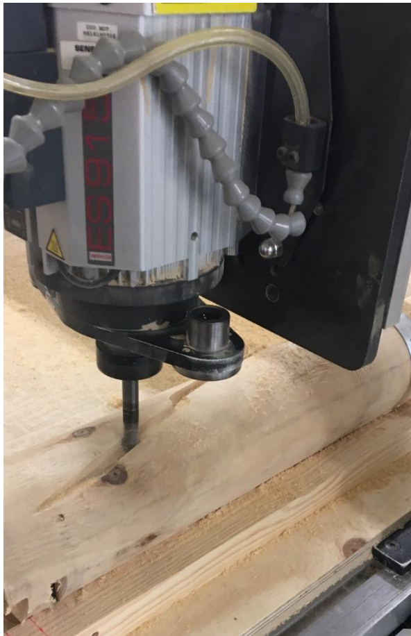
Figure 40. The geometry of the joint was coordinated with the machining constraints of the CNC router Photo by Author
