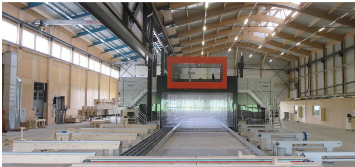
Figure 35. Timbercode facility in Gossau, note the size of the machining booth and dollies in the foreground. An overhead gantry supervision cabin has a clear acrylic floor which allows the supervisor to monitor the machining from above. Photos by Blumer Lehmann
