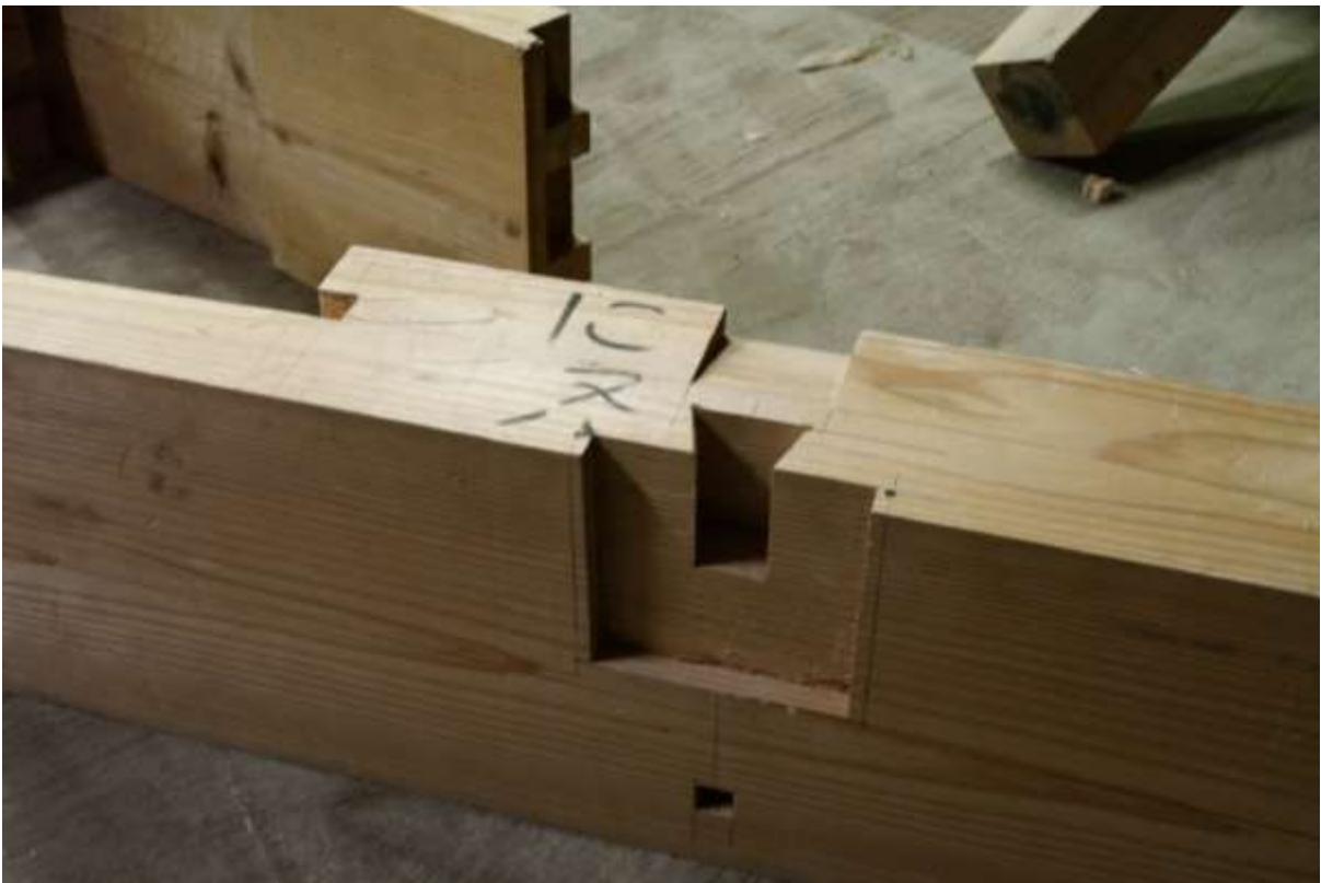
Figure 32 Marked framing members in Zgola's workshop. Photo: GA
