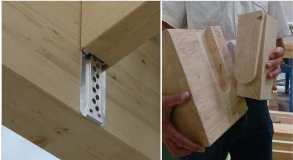
Figure 86 Rothoblaas Joist connector at the WCTE 2016 in Vienna (left) and a timber connection tested at the ETH, Zurich (right) Photo: GA
