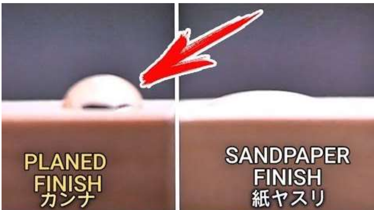
Figure 19 Water absorption of planed vs sanded finish Photo: Unknown
