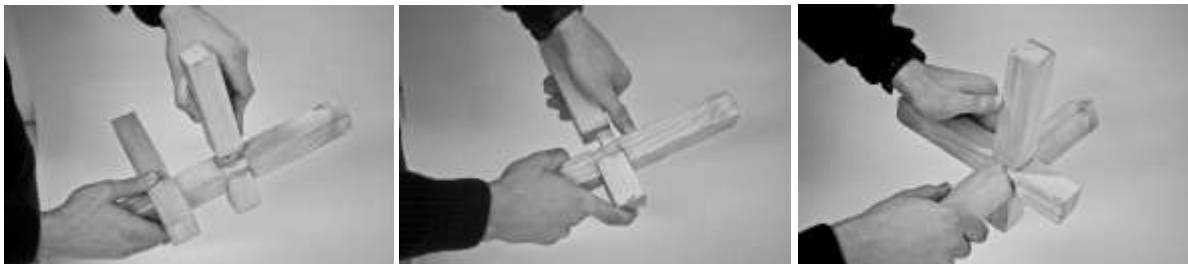
Figure 61 Assembly of the 'Chidori' joint Photo: https://slowerthanslow.files.wordpress.com/2014/12/chidori-joint-3.jpg
