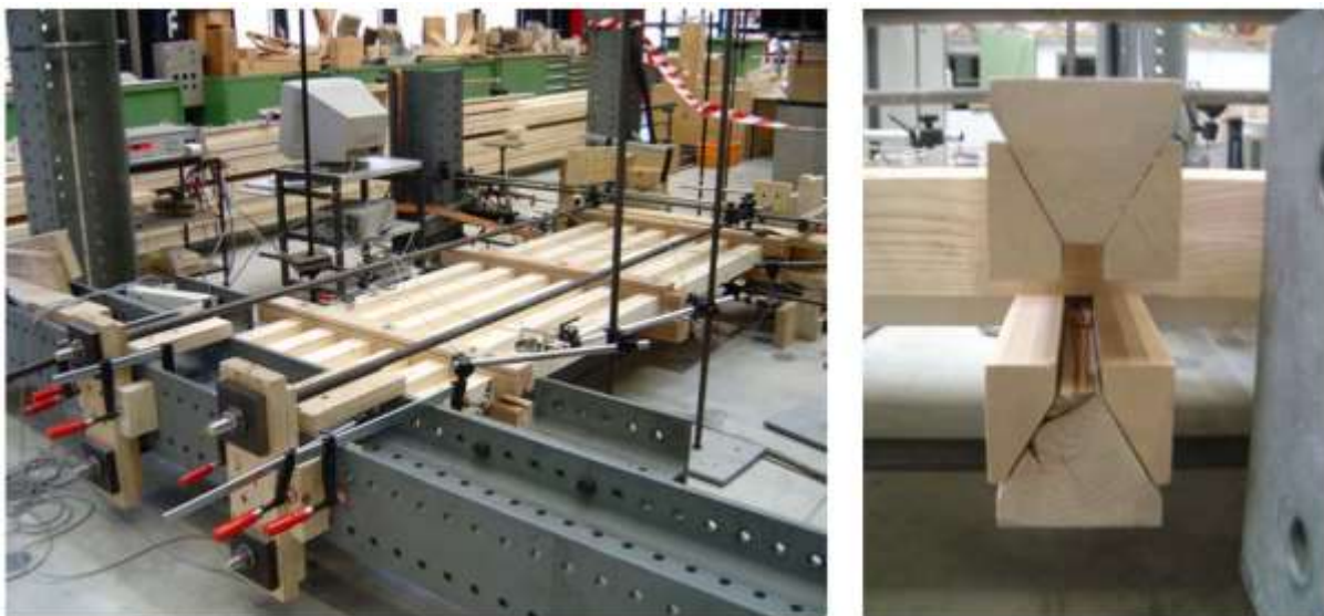
Figure 65 Shearing Test setup (left). Detail of staggered column - girths (right). Photo: T. Shiratori
