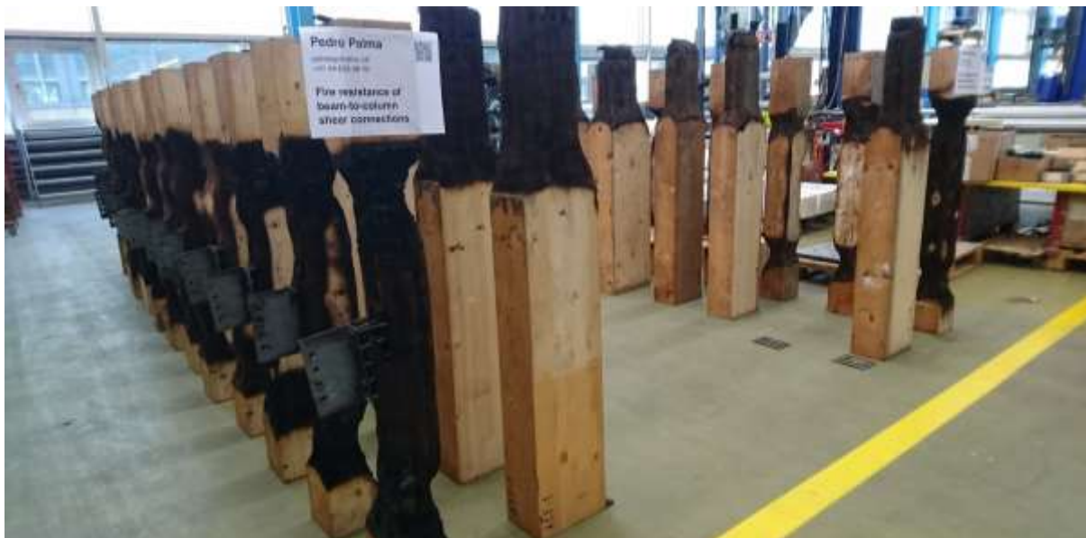
Figure 79 Fire resistance of Beam to Column connections [Pedro Palma, ETH Zurich]. Photo: GA
