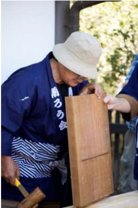
Figure 16 The carpenter aligns the blade and adjusts the cutting depth
