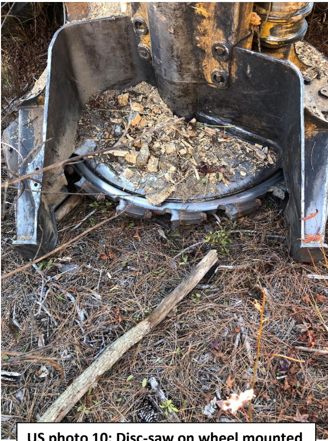
US photo 10: Disc-saw on wheel mounted feller buncher in southern pine harvesting operation
